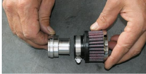
15. AIR PUMP ONLY: Rotate air pump fitting 90-degrees counter-clockwise.
