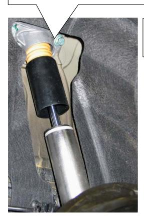
Mount the rear axle adjustment between spring and chassis, the original spring support is no longer used. You have to remove the rear axle adjustment to correct (screw up the threaded ring) the car height. Attention: Before the installation of the height adjustment perch the touching
