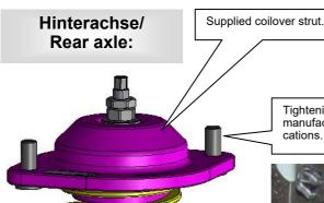
Tightening torque for the top fitting is 25 Nm (18 ft-lb). Please install the strut unit to manufacturers recommended settings regarding tightening torque and fixing specifi-
