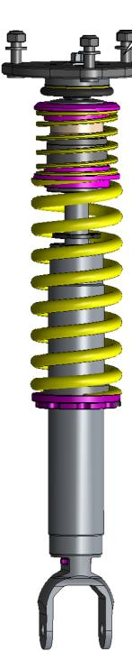
Tightening torque for the top fitting is 35 Nm (26 ft-lb). Please install the strut unit to manufacturers recommended settings regarding tightening torque and fixing specifications.
