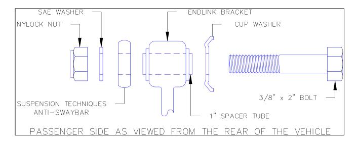
**11.** Refer to the diagram as to proper over/under steer adjustment.
