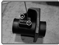
**8.** Secure and tighten the MAF sensor using provided M4 button head screws.
