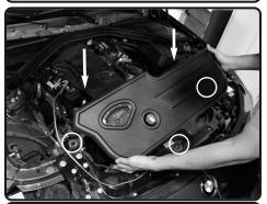
**20.** Install the air box assembly into the vehicle. Position the mounting points to the OEM location and secure.
