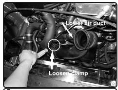
**5.** Use a 7mm nut driver to loosen the clamp on the lower turbo air duct. The upper air duct will be removed from the engine bay and no longer be used.
