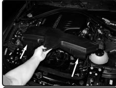
**4.** Firmy lift up on the OE air box assembly and remove it from the engine bay. Remove the engine cover.
