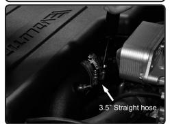
**21.** Connect the intake tube to the plenum. Secure and tighten using 8mm nut driver.
