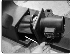
12. Now install the plenum assembly into the airbox.
