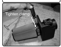
**9.** Install the filter to the plenum. Secure and tighten using 8m nut driver.
