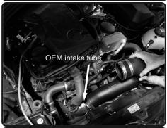
**17.** Install the new intake tube to the OEM intake tube.
