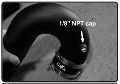
16. If vehicle is not equipped with vacuum line, remove the 1/8" brass fitting and install the provided 1/8" NPT cap. Secure and tighten.
