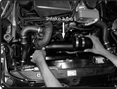
**18.** Position tube to sit in the center, and tighten the clamp.
