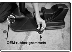
**14.** Remove the 2 factory rubber grommets from the OEM air box and install to the 2 larger holes on air box. These will be used to secure the injen evolution air box.
