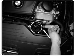
Use a 6mm nut driver and loosen the clamp on the MAF sensor housing located below the air box assembly. Also unplug the vacuum line
