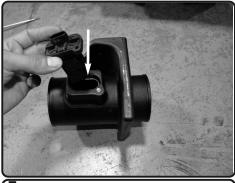
7. Install the MAF sensor into the new intake tube plenum.
