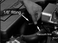
**22.** If vehicle is equipped with vacuum line, connect the vacuum line to the fitting. *If not equipped see step 16.*
