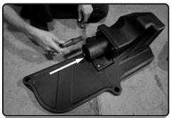
**13.** Now secure and tighten the plenum to the air box using 4 M6 screws with rubberized washers.
