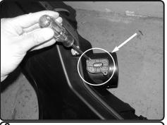
**6.** Use a torx driver and remove the two torx screws from the MAF sensor located on the OE air box assembly and then remove the MAF sensor from the MAF sensor housing.
