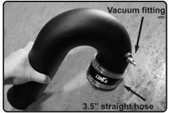
**15.** Please verify if vehicle is equipped with vacuum line, this fitting will be used. Install the provided 3-1/2" straight hose with clamps provided to tube.
