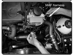
**19.** Pull back the MAF sensor harness away from oil cooler. This will allow to extend the MAF sensor harness.
