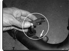
**26.** Loosen the two T25 torx screws holding in the temperature sensor and remove.
