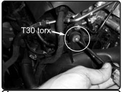
**4.** Loosen the T30 torx bolt on top of the intercooler pipe.
