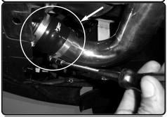
**34.** Secure the hump hose on intercooler and tighten using 8mm nut driver. Connect the hose and adjust. **Make sure the hoses are** properly adjusted and clamps are behind the bead. This will prevent hoses popping off the pipe
