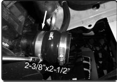
**28.** Now install the 2-3/8" x 2-1/2" hump hose to the intercooler. Make sure the 2-3/8" side is installed on intercooler.
