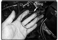
10. Check and verify the o-ring did not fall out, if so. use some grease and re-install to the groove cut out on the turbo. The grease will keep it from falling off.
