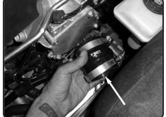
**14.** Install the provided 2-1/2" hump hose with clamps to the turbo adaptor.
