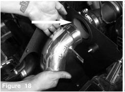
Install the intake tube and position to the hose and bracket to the vibra mount on heat shield.
