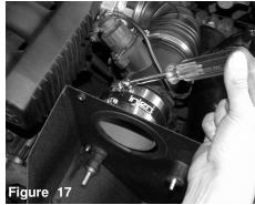
Position the hose to the hole cut out on the heat shield. Tighten the clamp on the MAF sensor only.
