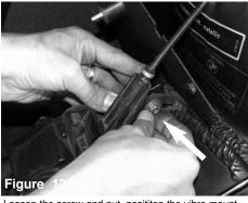
Loosen the screw and nut, posititon the vibra mount and secure using factory nut. Position the cable line through the slot cut out on heat shield.
