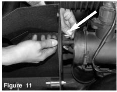
If equipped, Install the temperature sensor to the hole cut out on the heat shield. Secure using provided hex screw.
