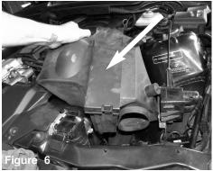
Carefully lift up and pull out the air box.
