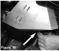
Secure the cover using the provided stainless M6 screws.
