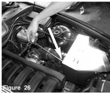
Secure and tighten the 3 screws using allen key.
