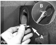
A) Install the vibra mount to the hole on the inside of the heat shield. B) With provided nut, secure the vibra mount and tighten using 10mm socket and ratchet.
