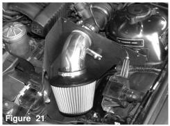
Make sure that the filter has clearance and not touching Install the vinyl trim to the cutout on the cover. anything. Loosen and position anything if necessary.
