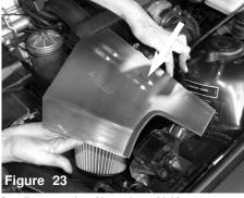
Install cover and position to heat shield.
