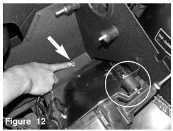
Secure the bottom of the heat shield using provided M6 nut to the thredded insert located on the frame of vehicle. Position the vibra mount to the Cruise control module.
