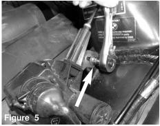
Loosen the the M6 nuts holding the cruise control module. Save the nuts for later install.
