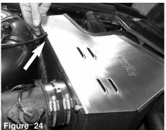
Make sure that the cable line is through the cut out on cover and heat shield.
