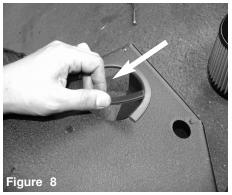
Attach the vinyl trim to the inside of the large hole on heat sheild.
