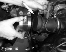
Attach the 3-1/8" straight hose with clamps provided to the MAF sensor.
