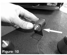
Attach the other vibra mount to the tab on housing. Secure using provided nut and washer. Tighten using 10mm socket and ratchet.
