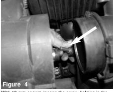
With 10 mm socket, loosen the screw holding in the temperature sensor and pull back.
