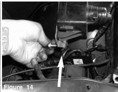
Use provided hex screw and washer and secure the bottom of the cruise control module using factory nut. Tighten using 10mm socket or wrench.
