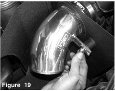
Position for the best fit and secure the bracket using provided washer and nut. Tighten using 10mm socket ance. or wrench.
