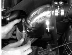
Install the filter and position for the best fit and clear-
