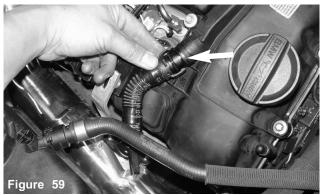
Connect the crank case line on the engine side.
