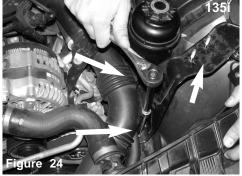
Loosen the 2 remaining nuts holding in the bottom of the bracket to the frame of vehicle. Pull harness away from bracket.
