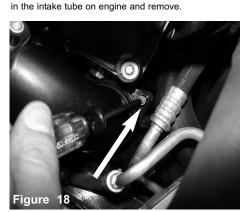
With T30 torx bit, loosen the screw holding in intake tube @ turbo housing.
