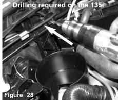
Applicable to the 135i only: Use a 1/4" drill bit to drill a hole through the composite cross member, the short bracket on the cup is used as a pattern.
