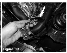
Remove the reservoir clamp from vehicle.
