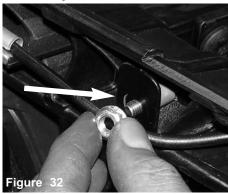
The m6 flange nut is used to tighten the reservoir bracket in place. **Note:** The 3/16" spacer between the bracket and cross member, used to support the bracket to keep it from distorting.
