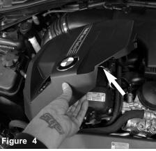
Carefully pull up and remove the engine cover.
