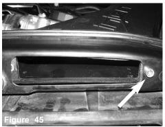
Install the injen power-scoop only to see how you will only be able to line up the 1 hole closes to the power steering resovoir bracket. Remove the screw.
