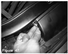
Install the factory scoop, secure the passenger side using the M6 button head screw and flange nut behind the core support.
