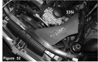
335i power-scoop and resovoir/air scoop bracket shown above. *Note: Remaining steps will be the same for both the 135i and 335i.*
