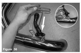
Install into the new lower assembly intake tube. Secure using the M4 button head screws provided.
