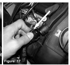
Carefully pull back the crank case fitting from the engine using a small flat head screwdriver.
