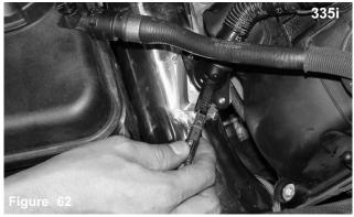
Connect the Crank case line harness.
