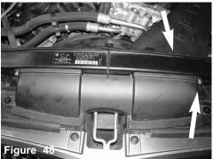
Position the injen power-scoop to the back of the core support, locate the 1 insert though the scoop. Secure the power-scoop using the M6 button head screw. Secure the plastic push clips to the factory scoop.
