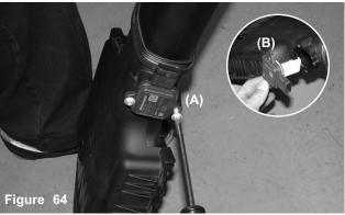
A) With t30 torx bit, loosen the 2 screws holding in the MAF sensor. B) Remove the MAF sensor.
