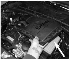
Lift and remove the upper half of air box out of vehicle.
