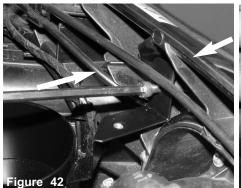
Make sure the spacer is used to preventing the bracket to distort. Tighten using allen key till bottoms out.
