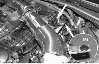
A) Attach the grommet to the hole on the bracket. B) Install the upper intake tube assembly into the vehicle and position to the tube and factory airbox engine fitting.
