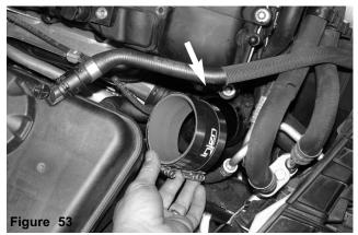
With clamps provided, install the 3" straight hose to the turbo housing.
