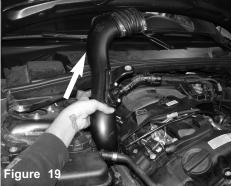
Carefully lift intake tube and slide back towards firewall and remove. *Make sure you remove the rubber gasket on turbo housing.*
