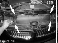
For the **335i** loosen and remove the 2 bolts and 2 plastic push clips holding in the primary 1 piece air scoop using t25 torx bit.
