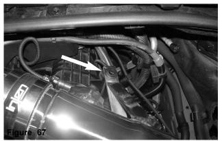
Make sure that the grommet is installed and seated properly as shown in above photo.
