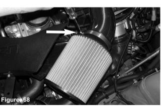
Install air filter to the tube and tighten and secure
