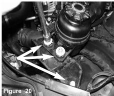
Loosen the 2 nuts holding in the power steering reservoir. Also, loosen the 10mm screw holding in the bracket.
