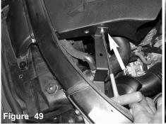
Install the Air scoop bracket to the power-scoop. secure using M6 button head screw.
