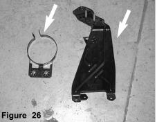
Once removed, you should have completly removed the power steering reservoir bracket and clamp from vehicle.
