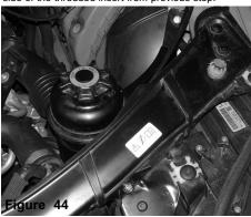
Install the resovoir into the cup and secure. **Note:** Make sure the resovoir bottle sits all the way down and tight.
