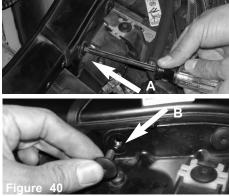
A) Loosen the bolt on left side of core support holding in headlight using T30 torx bit. B) Remove the bolt from vehicle.
