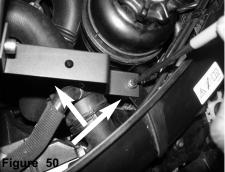
Position the bracket to the power steering resovoir bracket thredded insert. Secure using the remaining M6 button head screw and tighten. This will allow for support of the power-scoop. (NOTE: you should have 1 remaining flange nut, please discard)
