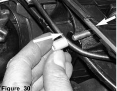
The 3/16" aluminum spacer is slipped over the m6 x 35mm bolt used to secure the reservoir bracket.
