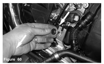
From step 15, use the factory bolt and provided fender washer to secure the bracket on engine. *Note: Make sure you use the fender washer.*
