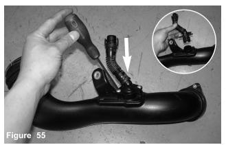
With t30 torx bit, loosen the 2 screws holding in the crank case line. Carefully pull out and remove.
