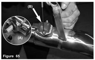
A) Install the MAF sensor into the new intake tube. B) Secure the MAF sensor using the provided M4 button head screws. Page 7 of Part# SP1126
