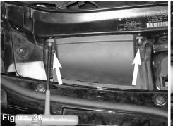
Secure the passenger factory side scoop using the M6 button head screws and 2 flange nuts behind the core support.
