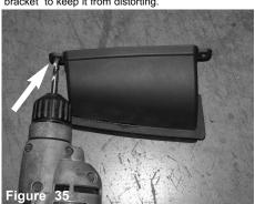
Drill all the 4 holes out to 1/4" on the factory scoops to make the M6 screws able to pass through.
