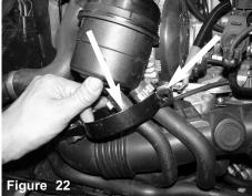
Carefully pull the clamp apart, and silde making the 2 lines pass the clamp.
