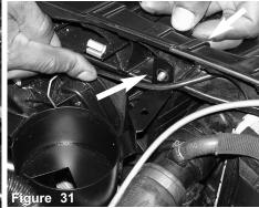
The m6 x 35mm hex bolt is inserted through the cross member, and into the 3/8" aluminum coupler. The aluminum coupler is used as a back support for the reservoir bracket as shown in figure 28.
