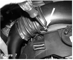
Loosen the clamp on intake tube using 7mm nut driver.
