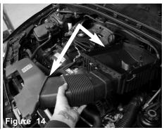
Lift and pull up the lower air box assembly from the 3 grommets attached to the engine and remove.
