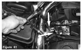
Secure the bracket and slide the slot on bracket forward so it stops and tighten using 10mm socket and ratchet.
