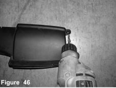
Drill both holes out to 1/4" on the factory scoop to make the M6 screws able to pass through.
