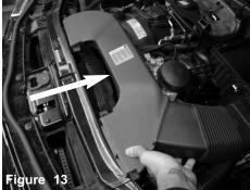
Lift up and pull back the the lower primary air scoop assembly.
