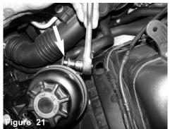
With 10mm ratchet and extension, loosen the screw holding in the reservoir clamp.
