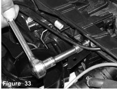
A 10mm socket and ratchet is used to fasten the flange nut to the m6 bolt.
