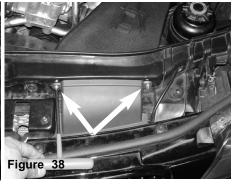
Tighten the 2 screws using allen key and secure. **Note:** *This does not require the use of the air scoop bracket only, for the 335i.*
