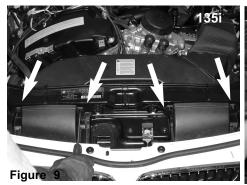
For the **135i** only loosen and remove the four bolts holding the primary air scoops in place using t25 torx bit.
