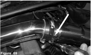
Position for BEST POSSIBLE FIT. Note: This may need a lot of adjustment with both tubes. Make sure that the hood has clearance and the tube is not touching the fuel line below. Tighten all clamps using 8mm nut driver.
