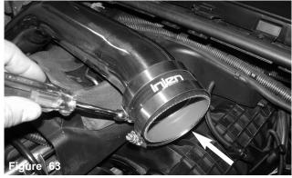
Install the 3" straight hose with clamps provided and attach to the end of the intake tube. Tighten on the tube only.
