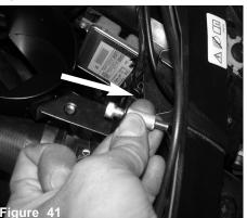
Install the M6x35mm bolt through bracket, now install the spacer to the bolt. Position the bolt to the back side of the thredded insert from previous step.
