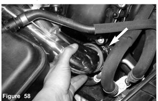
Position the tube and make sure it fits secure. Do not tighten.
