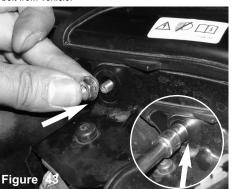
Use provided flange nut and secure the bolt. Tighten using 10mm socket and ratchet.
