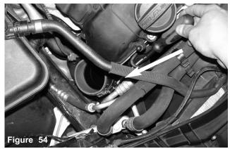
Secure the clamp on the turbo housing only using 8mm nut driver.
