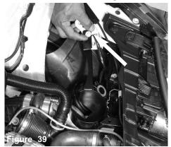
The stock m6 bolt is used to fasten the extended bracket located on the new power steering cup.
