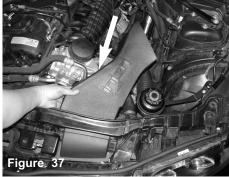
Install the driver side factory scoop, position the injen power-scoop to the back of the core support, locate the 2 inserts though the scoop. Secure the powerscoop using the 2 remaining M6 button head screws.
