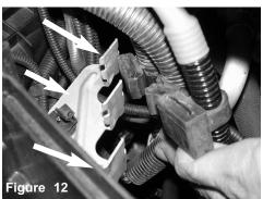
Pull back the 3 harness lines attached to the lower air box assembly.
