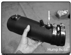
**13.** Install the 1/8" NPT fitting, to the insert on intake tube and secure. Install the 3-1/2" hump hose with clamps provided to the intake tube.
