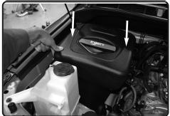
11. Place the Injen air box assembly into the engine bay and line up the pegs below the Injen air box to the vibramounts.
