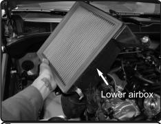
**7.** Remove the bottom half of the airbox out of the vehicle.
