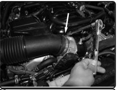
**2.** Lift up firmly to remove the engine cover. Loosen the clamp on throttle body using 10mm socket and ratchet.
