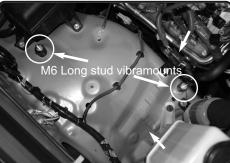
**10.** Using the OEM mounting locations, install provided long stud vibramounts to the thredded inserts. *Make sure the long stud is facing up. short side is secured.*
