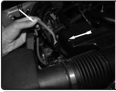
**4.** Disconnect the MAF sensor harness. Pull harness from the air box.
