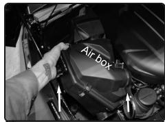
**4.** Carfully lift up and remove the airbox from the vehicle.
