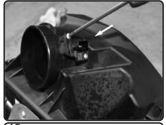
**15.** Loosen the 2 screws holding in the temp sensor using T25 torx bit and remove from air box.
