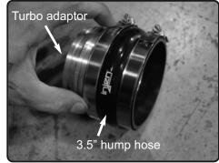
**8.** Install the 3.5" hump hose to the turbo adaptor with clamps provided. Tighten clamp on the adaptor only.
