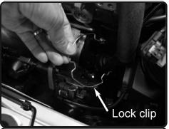
**5.** With a flat head screw driver, pull back the lock clip on the turbo. Slide out intake tube from turbo. Save lock clip for later install.
