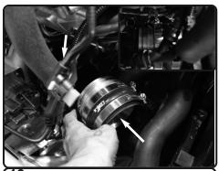
**13.** Install the turbo adaptor assembly into the vehicle. slide on to the turbo.
