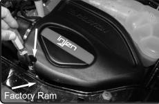
**12.** install the air box assembly into the vehicle. Secure using OEM screw. Make sure the nipple fitting on back side of injen airbox is seated in the OEM grommet on fender well.
