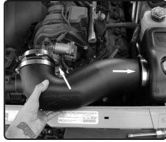
**16.** install the intake tube assembly into the vehicle and position.
