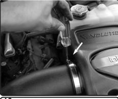
**18.** Secure the clamp on filter using 8mm nut driver.
