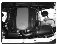
**1.** Stock air intake box and air intake duct shown above.
