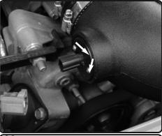
**20.** once seated, rotate the sensor and secure.
