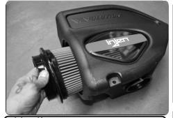
**11.** 1)Insert twist lock filter to the air box. 2)Once seated, rotate in either direction 1/4 turn till filter locks.
