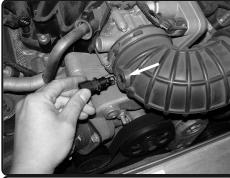
**4.** Firmly pull and remove air temperature sensor out of factory air duct.
