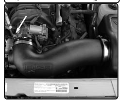
**17.** secure the tube and position for best fit. Tighten clamp on Throttle body.
