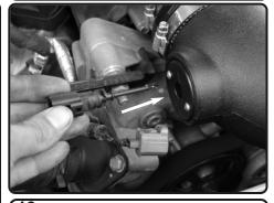
**19.** install the Temperature sensor into the adaptor. Re-connect the Harness.
