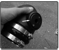
13. install the temp adaptor to the tube.
