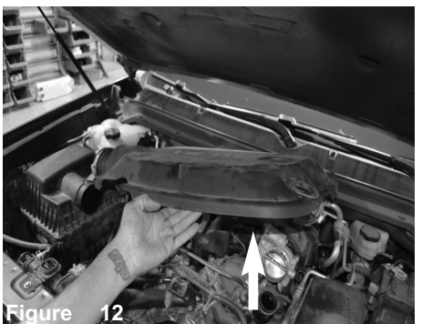
Figure 8 With 10mm socket and ratchet, loosen the screw on the back of the engine cover and remove.
