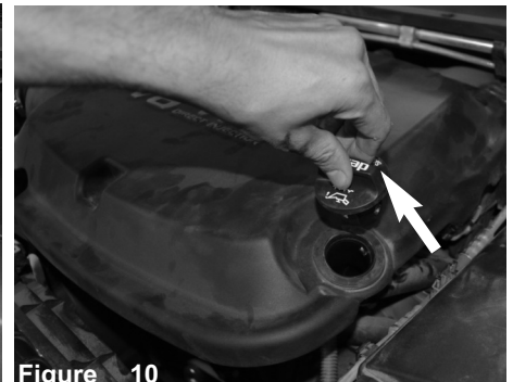
Figure 10 Remove the oil cap.
