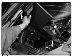
13. Install the heatshield into vehicle. Front tab will fit on radiator support.
