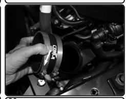
**20.** Install the provided 4" straight hose with clamps to the plastic intake tube. Tighten clamp on the plastic tube only.
