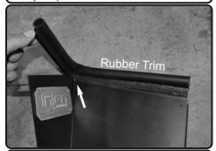
**9.** Intall the provided Rubber trim to the top of the heatshield. Notch corner with pliers/cutters for easier installation.
