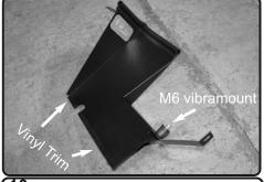
**10.** Install the provided Vinyl trim pieces to the bottom of the heatshield. Install the M6 vibramount to the Thredded insert on heatshield.
