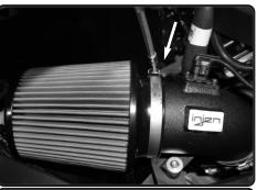
**26.** Secure and tighten using 8mm nut driver. Re-adjust if you need to and retighten intake tube.
