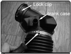
**5.** With a flat head screw driver, pull back the lock clip on the turbo. Slide out intake tube from turbo. Disconnect the crank case line on the intake tube by depressing clip. With flat head screwdriver, break the security clamp loose.
