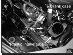
**8.** Re-install the plastic intake tube into the vehicle. Re-connect Crank case line. Make sure you hear a click, tug on tube to make sure the tube is secured to turbo and will not come off.
