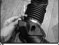
**6.** Remove the security clamp from intake tube.,
