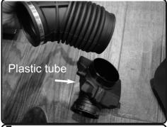
7. Remove the intake tube from the hard plastic intake tube. Make sure the Lock clip is seated correcty in the intake tube to allow the tube to secured properly to turbo.
