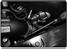
**23.** Tighten the clamp on the intake tube using 8mm nut driver.
