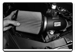
**25.** Install the air filter to the intake tube.
