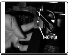
**15.** Secure the heatshield tab to the radiator support using M6 screw and M6 nut. Secure and tighten using 10mm wrench or ratchet.
