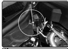
**12.** Loosen the T30 torx screw located near Postive battery terminal. Save bolt for later install.
