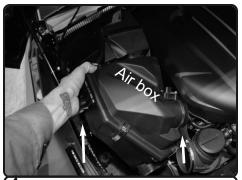
4. Carfully lift up and remove the airbox from the vehicle. Note: Next photo intake tube was removed for easier look at intake tube and for photos.
