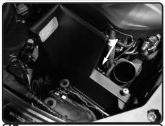
**17.** Complete heatshield assembly installed. Tighten all screws and secure.
