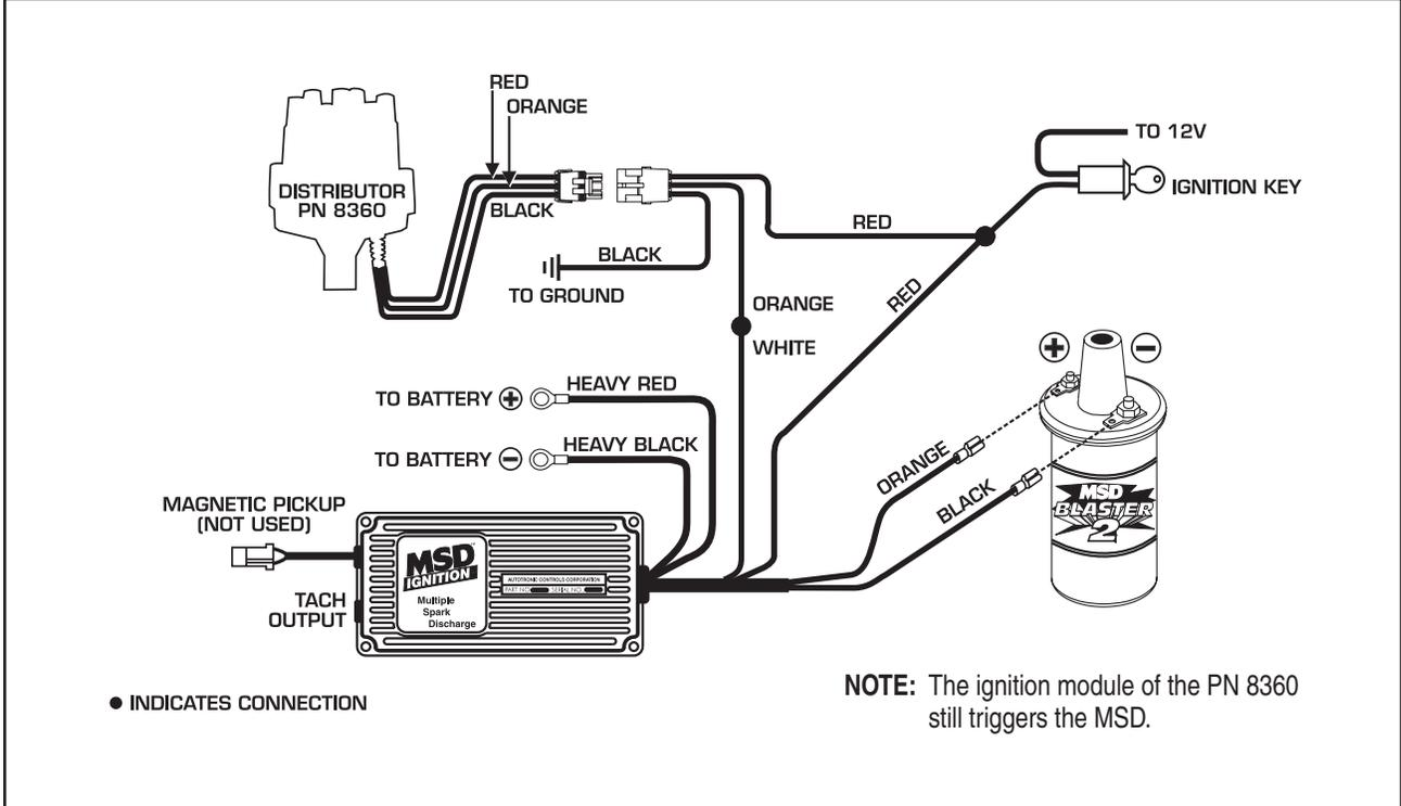
**MSD SYSTEMS With an MSD Timing Control (points or amplifier).**
