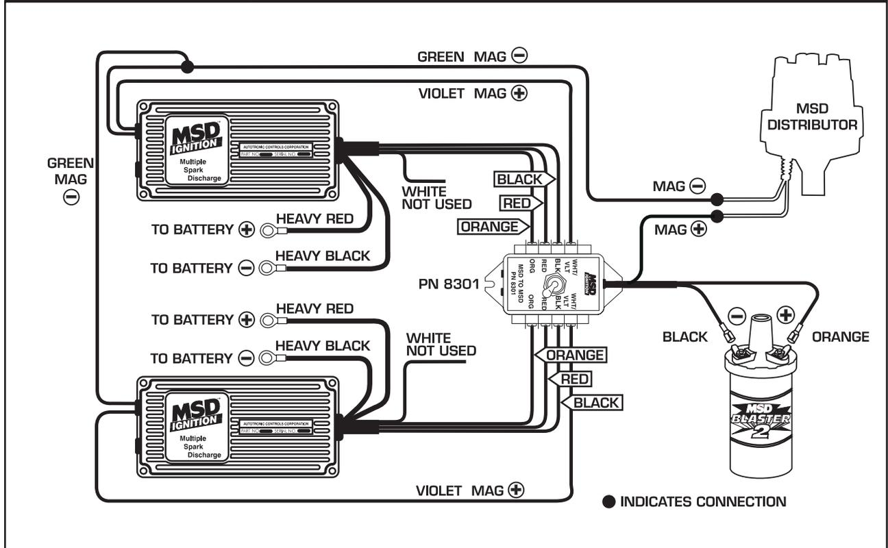
**MSD SYSTEMS Wiring a Complete Dual MSD Ignition Setup.**
