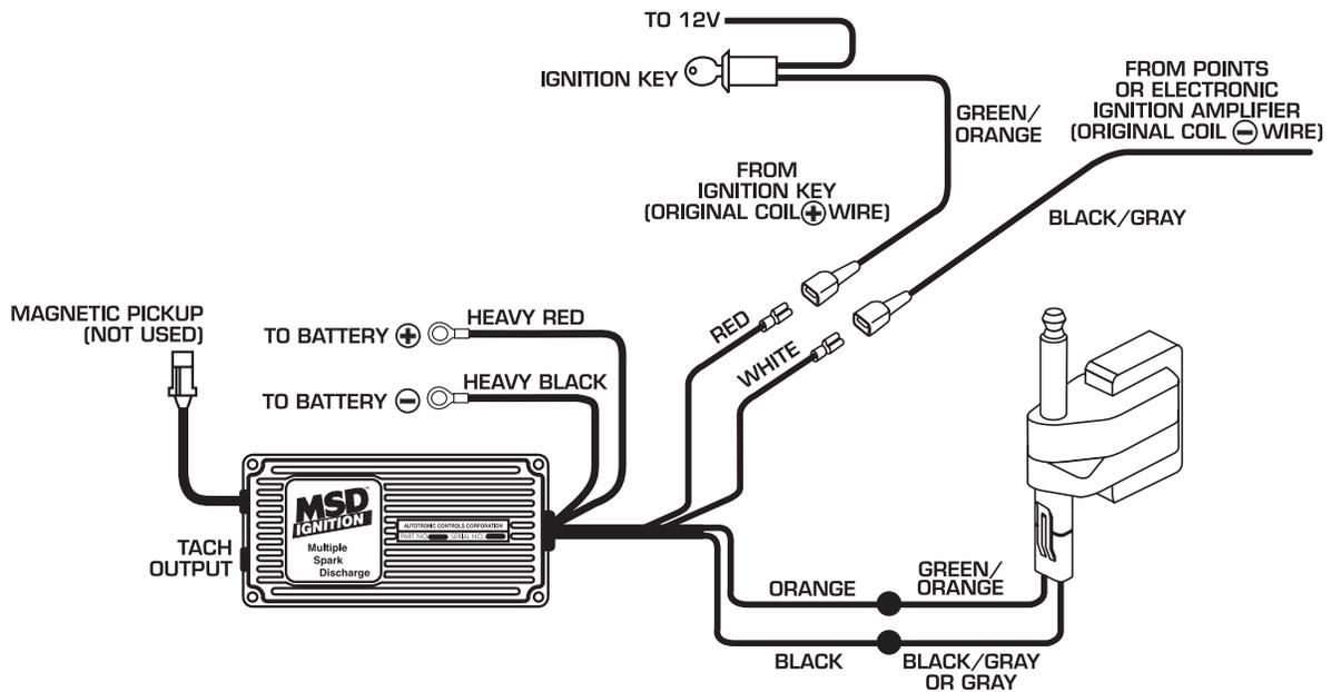
**NOTE:** Original coil wiring will be cut.
