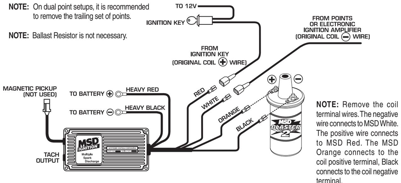
**MSD SYSTEMS** Installing to an MSD Distributor/Crank Trigger.
