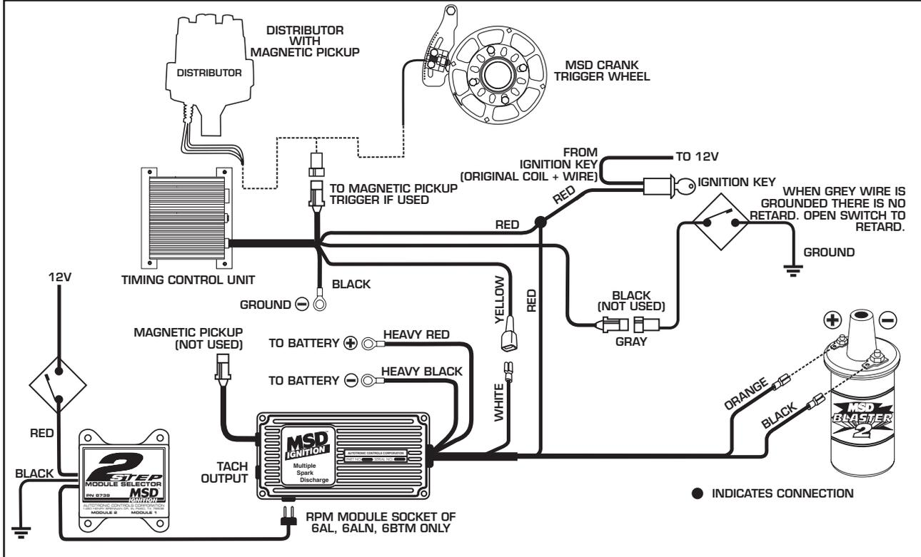
**MSD SYSTEMS Wiring Dual MSD's with PN 8301 Switch.**
