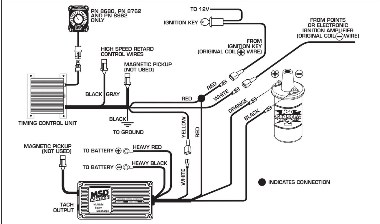
**MSD SYSTEMS Typical Drag Race Setup with Timing Control and Two Step Selector.**
