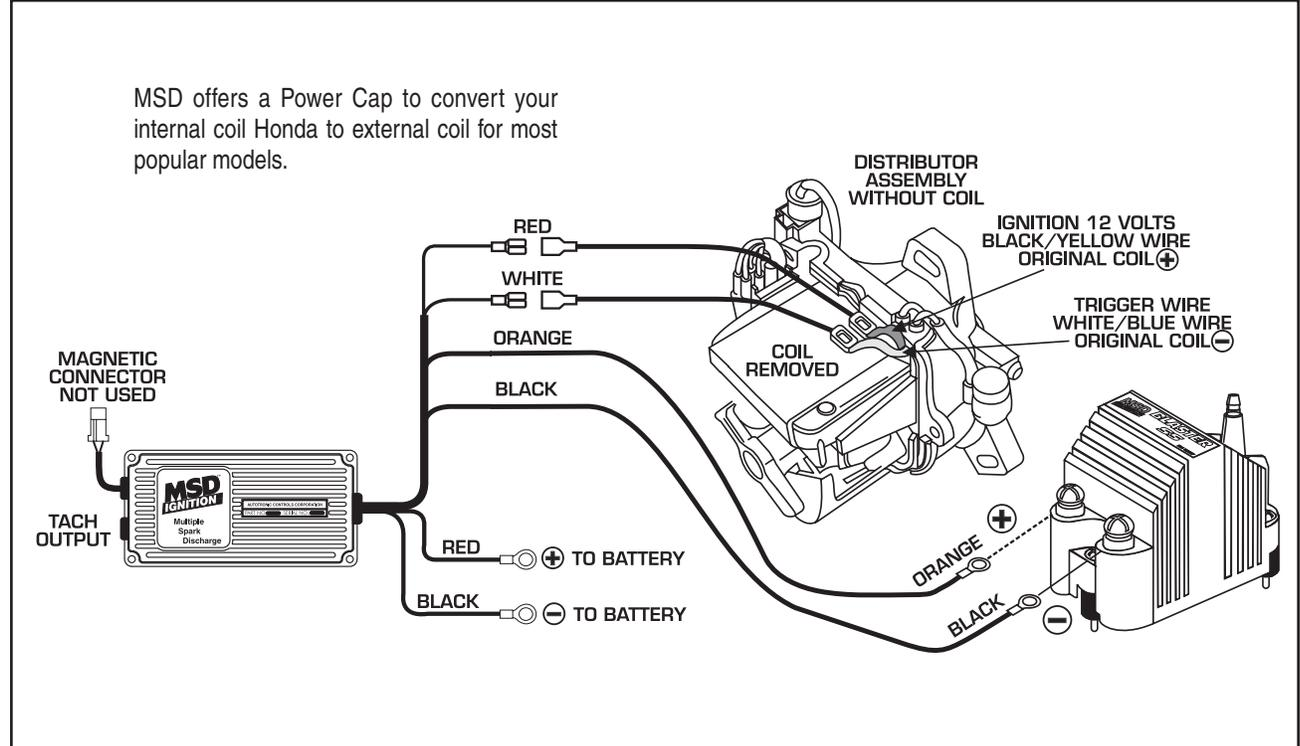
**HONDA IGNITIONS Wiring a Factory External Coil Honda/Acura .**
