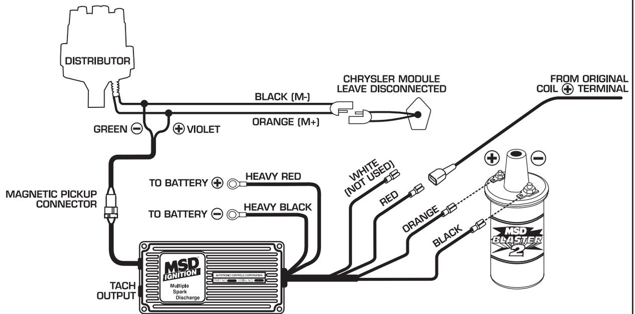
**CHRYSLER IGNITIONS** Wiring a Late Model Dodge with 2-pin connector.
