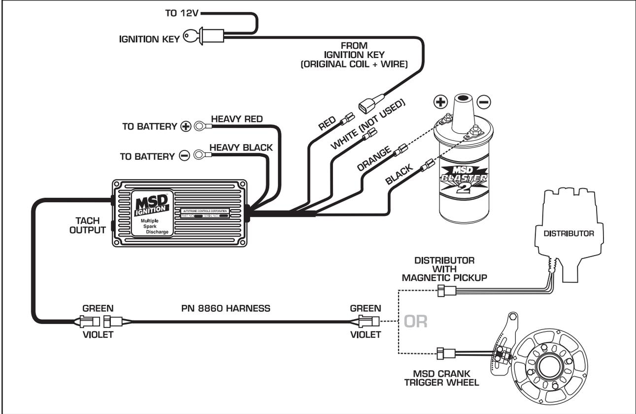
**MSD SYSTEMS** Installing to an MSD Distributor PN 8360.
