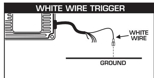
Figure 8 Checking for Spark with the White Wire.
