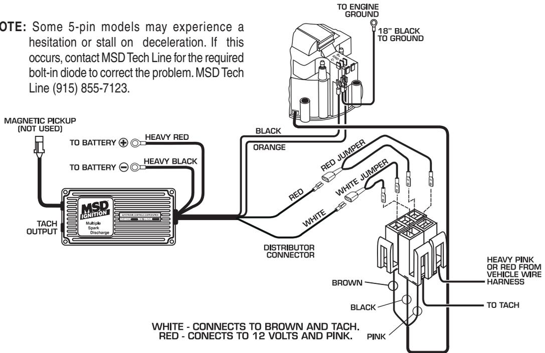
**FORD IGNITIONS Wiring a Ford DuraSpark using White Wire Trigger.**
