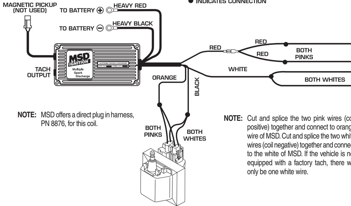
**GM IGNITIONS Wiring the 1996 and up single connector coil without harness.**
