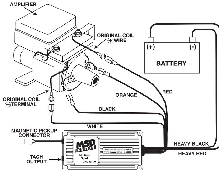
**AFTERMARKET COMPONENTS** Wiring a Mallory 9000 Series using Magnetic Pickup.
