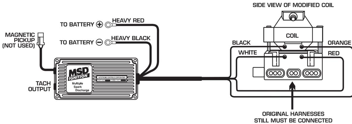
**HONDA IGNITIONS** Wiring a Honda with Internal Coil.
