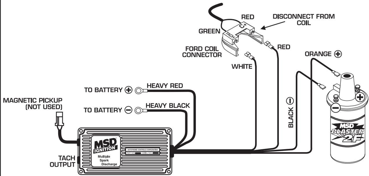
**FORD IGNITIONS Wiring a Ford DuraSpark using Magnetic Pickup Trigger.**
