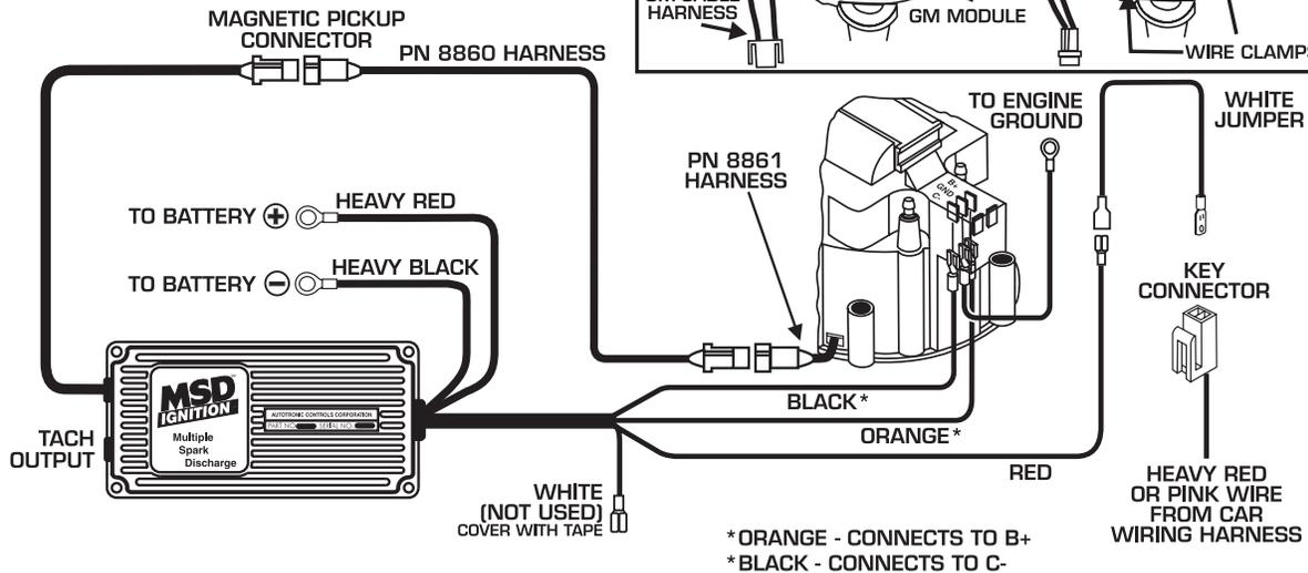
**GM IGNITIONS Wiring an HEI 5 or 7-pin Module (Amplifier Trigger).**
