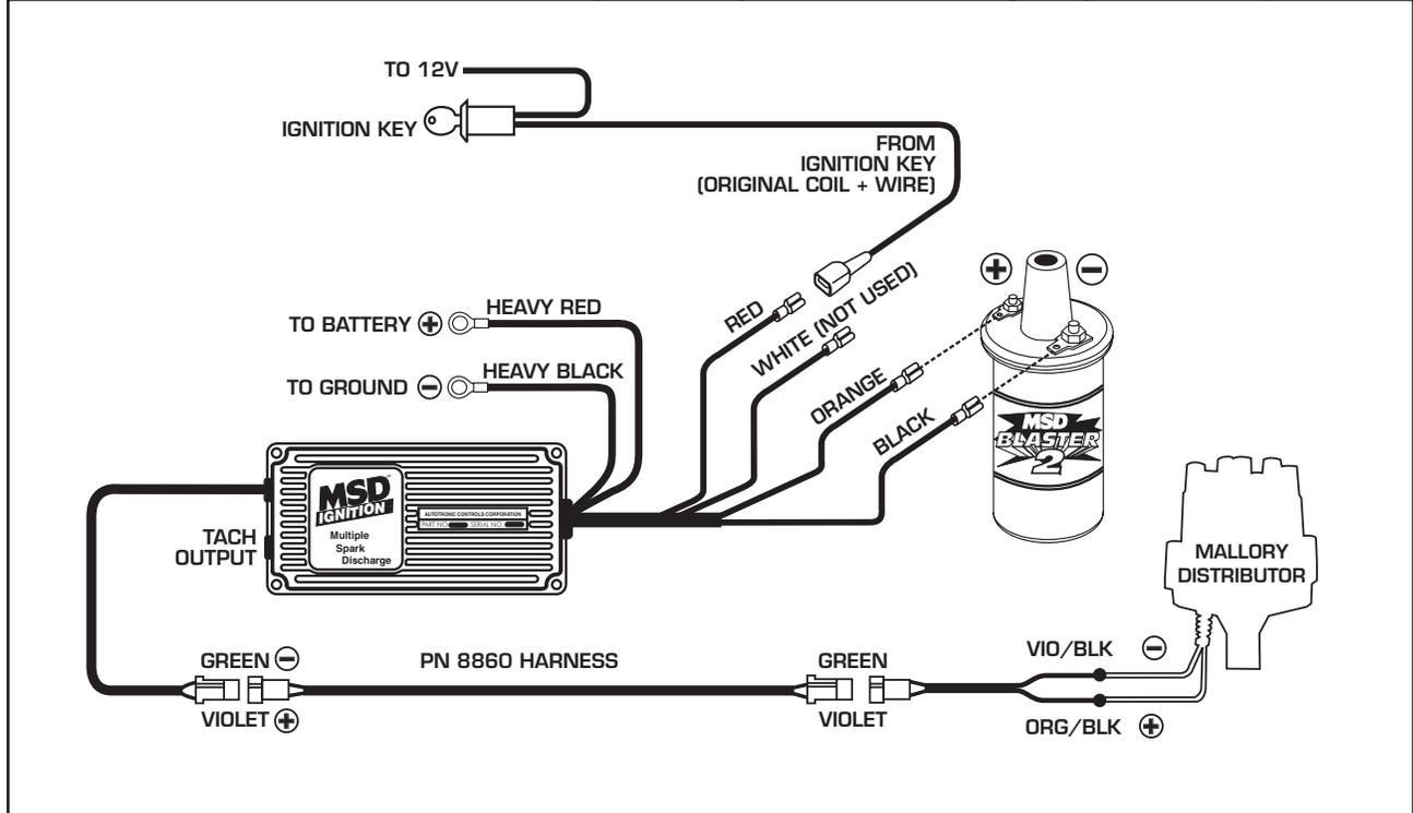
**AFTERMARKET COMPONENTS** Wiring a Mallory Unilite or 9000 Series using Points Trigger.
