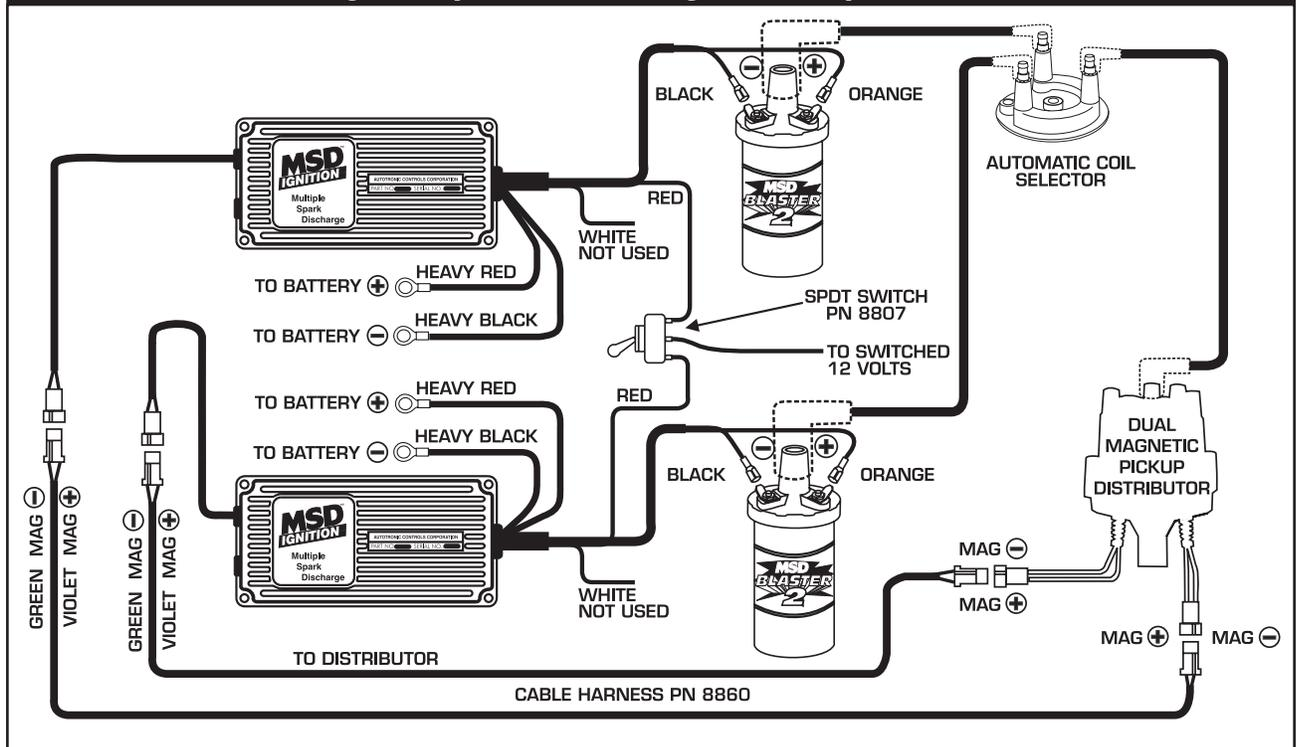
**GM IGNITIONS Wiring a Dual Connector Coil.**
