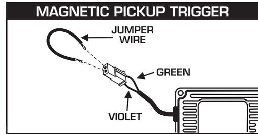
**Figure 9 Checking for Spark with Magnetic Pickup.**
