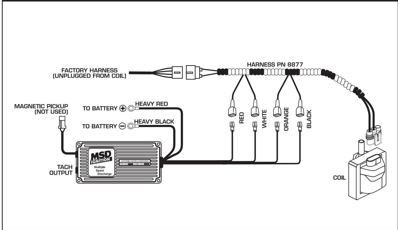
**GM IGNITIONS Wiring with an MSD Wiring Harness and a Timing Control.**
