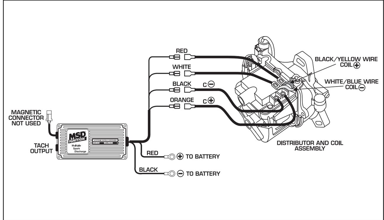
**HONDA IGNITIONS** Wiring a Honda with a Blaster Coil and Power Cap.
