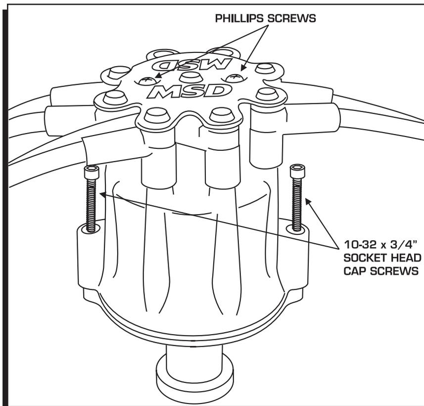
**Figure 1 Installing the Wire Retainer.**
