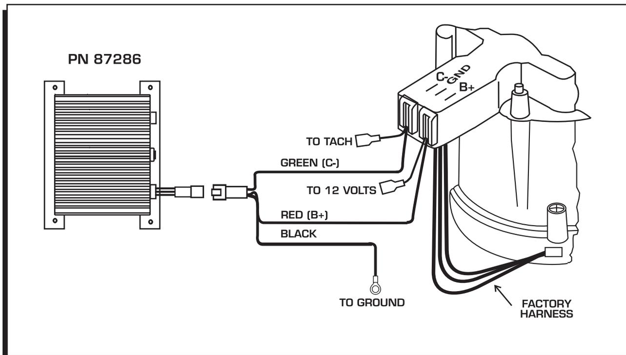
**Figure 2 Wiring the PN 87286.**
