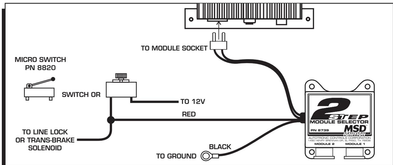
Figure 1 Basic Two Step Module Selector Installation.
