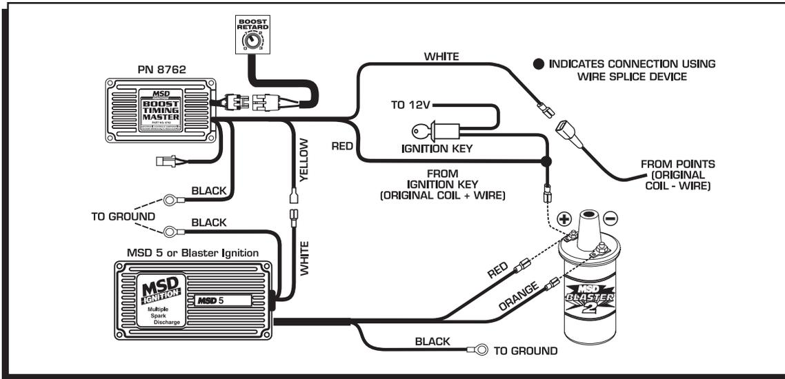
Figure 4 Wiring for MSD-5 / Blaster Ignition.
