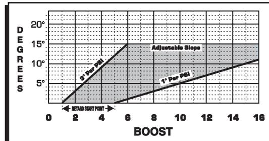
Figure 3 Setting the Timing Adjustments.
