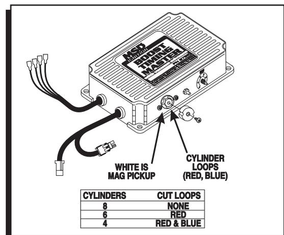
**Figure 1** Selecting the Cylinders or Trigger Pickup.
