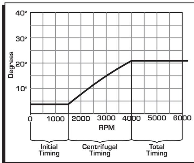
Figure 1 Typical Timing Curve.
