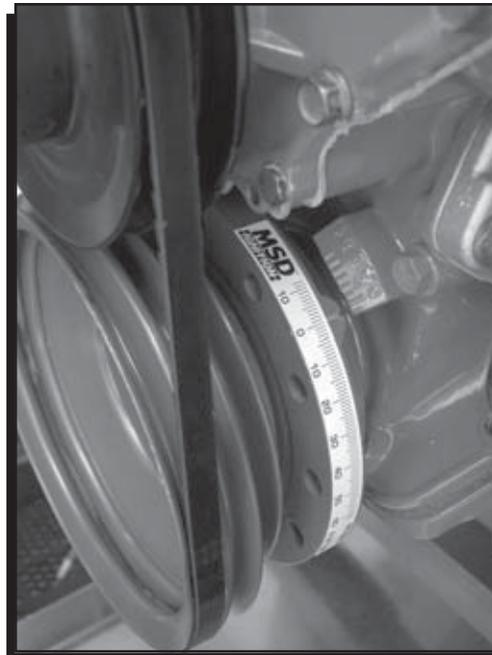
Figure 2 The Timing Tape Installed.
