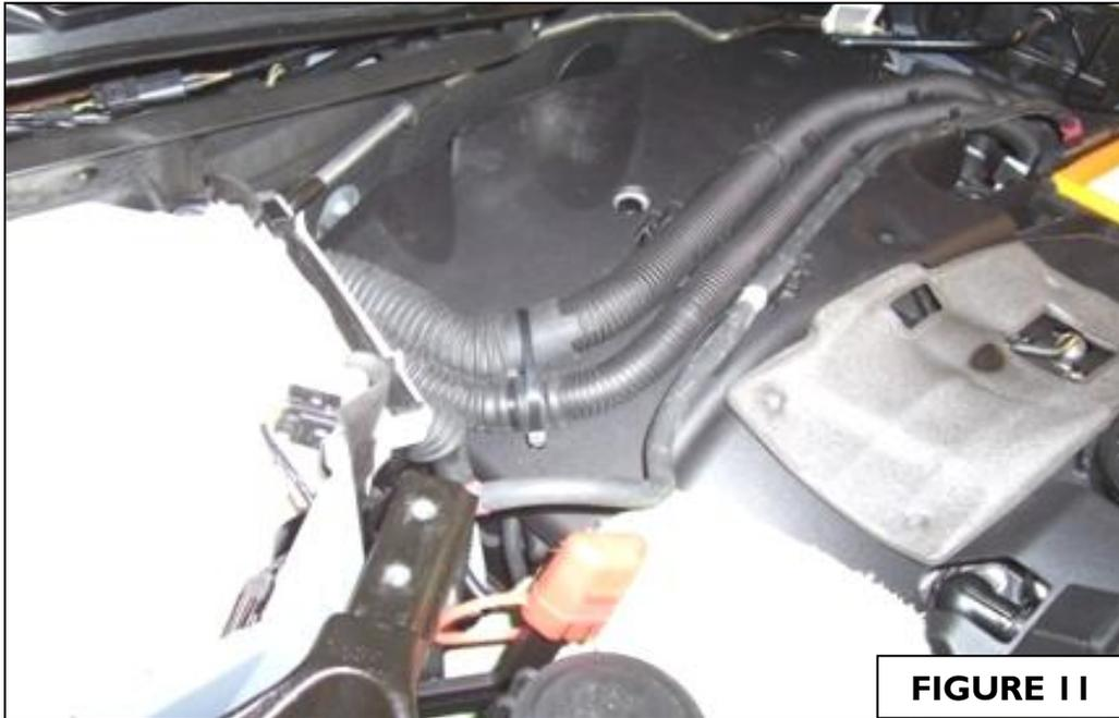
14. Reinstall wire harnesses and rubber holders to coil cover.
