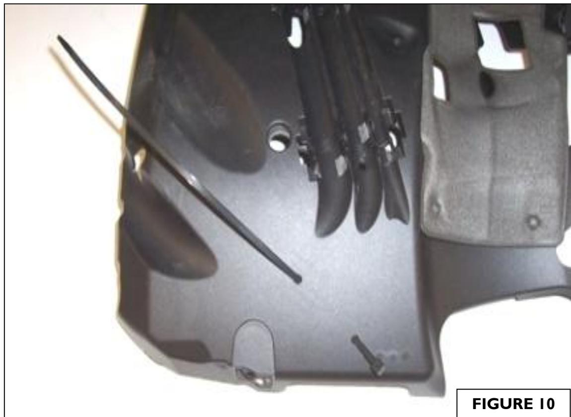
13. See Figure 11. Reinstall coil cover with cable tie under wire harnesses. Place wire harnesses inline with cable tie on coil cover and attach cable tie. Make sure wire harnesses are positioned like photo to prevent cable tie from damaging wire harnesses.
