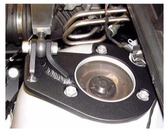
6 Now, secure endplates to strut towers. Nuts should be tightened to 18 ft-lbs.
