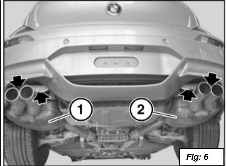
6. Remove the rubber hangers with mounts from the stock mufflers by pulling them off the wire hangers on the mufflers.
