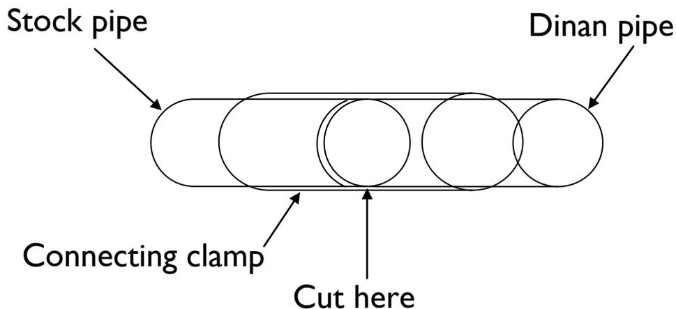
2. Check to see if your marks are about 1.75" from the insulation on the pipe close to the differential. See figures 2, 3 & 4.
