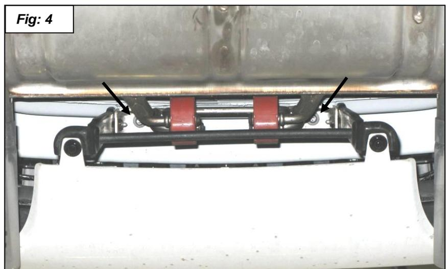
7. Look at step 10 before doing this step. Remove the two nuts holding the side hangers on each side of the car as shown in figure 3 (one side is shown). Remove the grounding straps.
