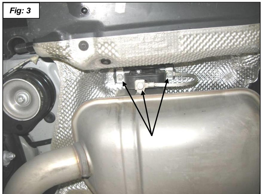
5. E93 ONLY: Remove the underbody reinforcement straps.
