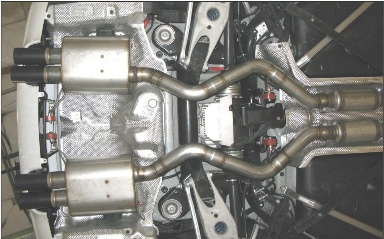
2. The exhaust tips are different lengths between the E90 & E92/E93 Dinan M3 exhausts. Measure the tips to confirm that you have the correct mufflers:
