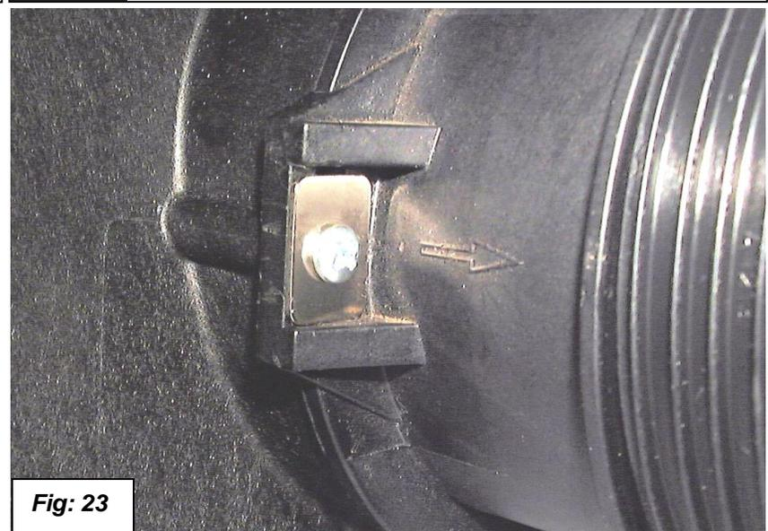
29. Install the filter onto the Dinan lid at a 97° angle and tighten clamp. See figure 24.
