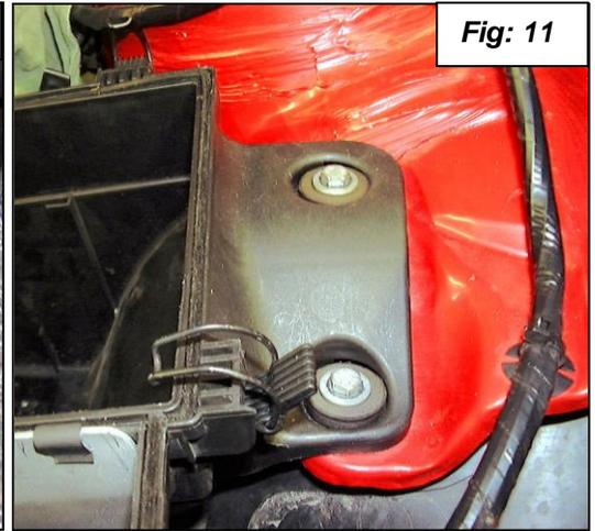
11. Pry back clips for air flow meter and separate AFM from airbox lid, **be careful not to damage the grid on the AFM.** (The airbox lid will not be reinstalled on the car). See figure 12.
