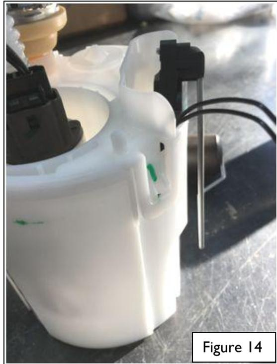
14. Identify the stock fuel line that runs between the center of the fuel filter and pressure regulator. This line will be removed.
