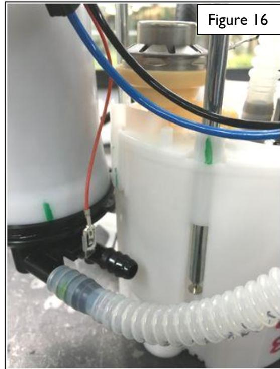
16. Locate the Dinan Internal Hose Assembly #2. This line and tee assembly replaces the fuel line you just cut off. Attach the short hose of the tee to the fuel filter with the tee pointing upwards (see Figures 17 and 18).
