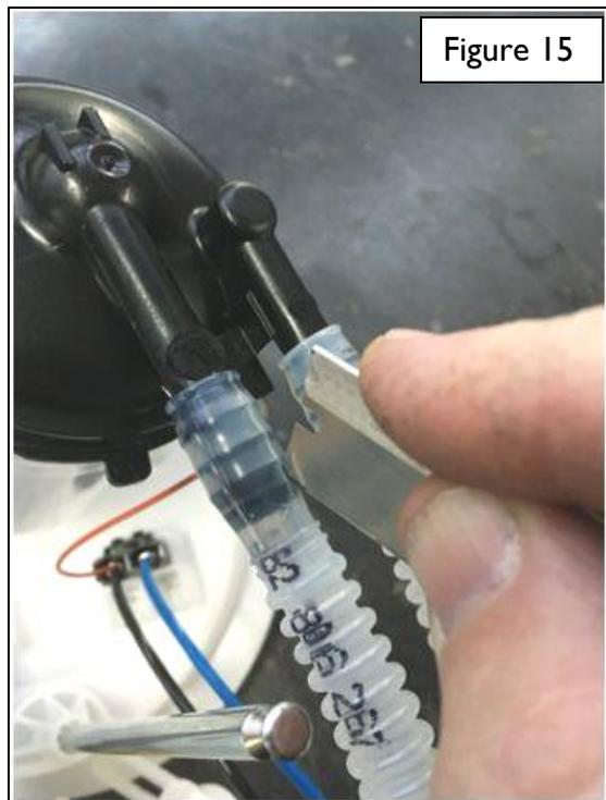
15. After removing the stock fuel line, reinstall the fuel filter half of the assembly onto the lower cup section using the spring and attaching it with the small E-clip (see Figure 16).
