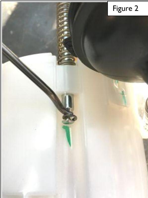
6. Pull the upper filter section of the assembly upwards until the 2 legs are free of the lower pump section. Do not lose the spring (see Figures 3 and 4).
