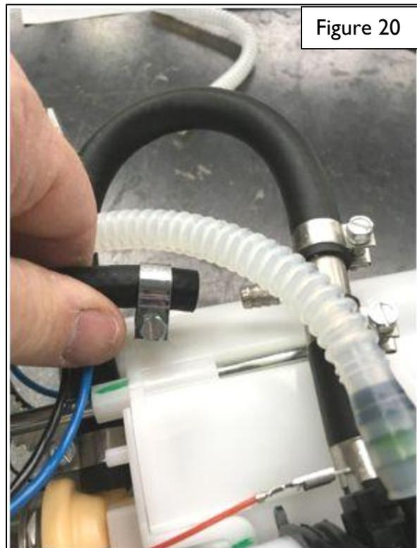
19. Tighten all the hose clamps and be sure all the wire plugs are connected and seated.
