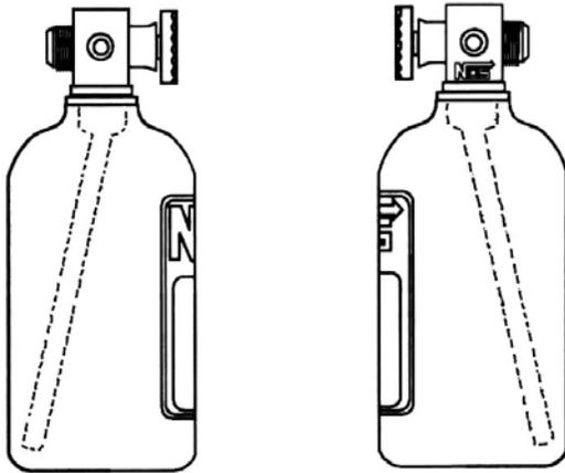
**Figure 4 Nitrous Bottle Mounting Orientations**
