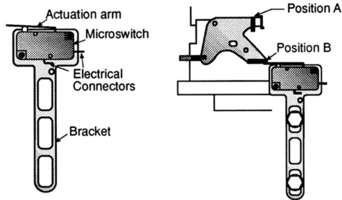
3. Install the NOS arming switch in the vehicle interior, within easy reach of the driver.
