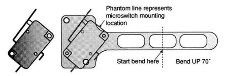
**NOTE:** The microswitch may be mounted to the bracket in a variety of positions and on either side of the bracket. The bracket may be bent to suit the application.
