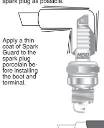
Wiggle the boot to see if the connector is gripping the spark plug terminal tightly. If any play is felt, replace the boot and connector.
