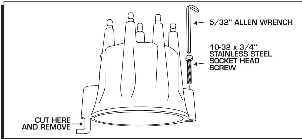
**Figure 10 Optional Installation by Bolting the Cap Down.**
