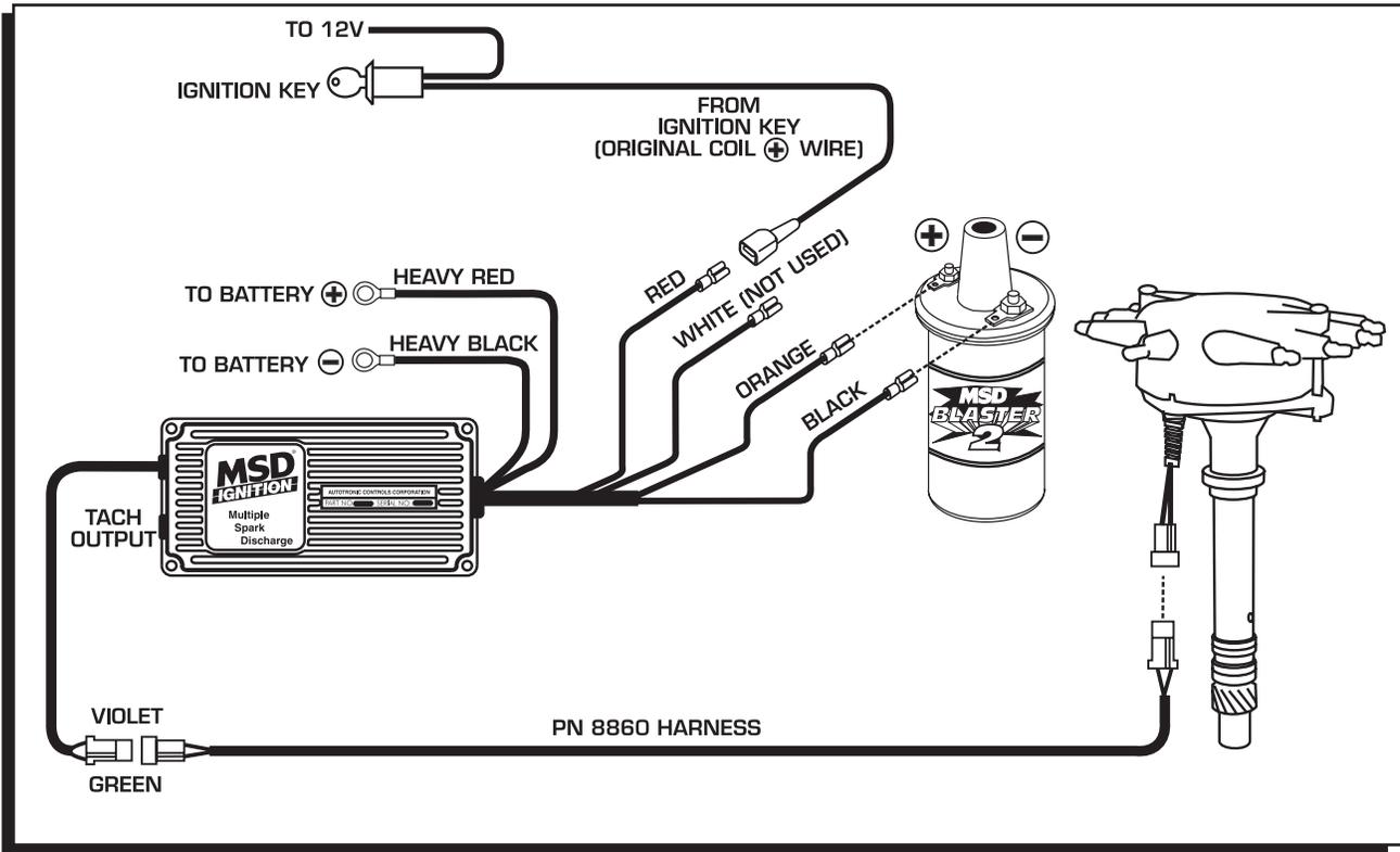
Figure 10 Wiring to an MSD 6-Series Ignition Control.
