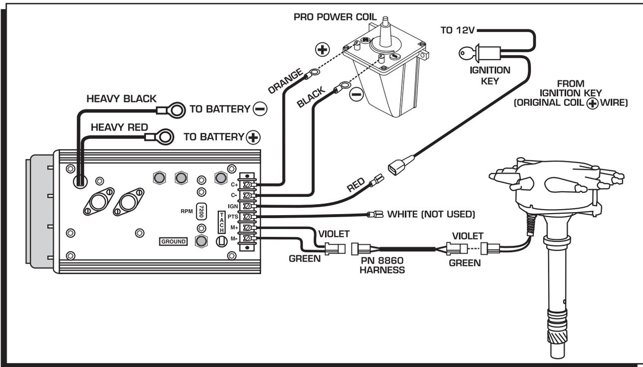
Figure 11 Wiring to an MSD 7-Series Ignition Control.
