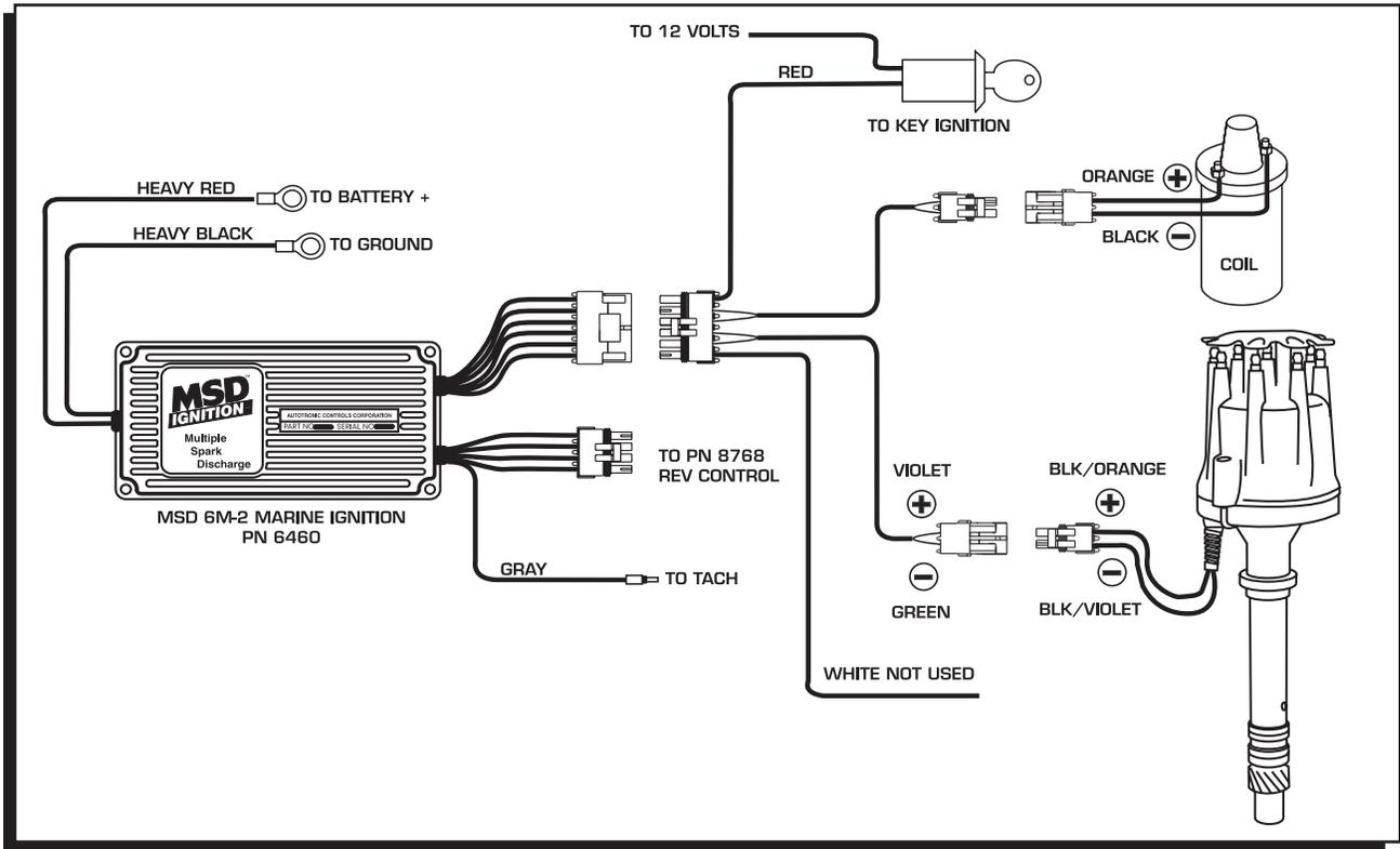
Figure 12 Wiring to an MSD 6M-2 Ignition Control.
