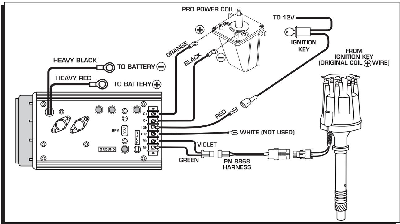
Figure 13 Wiring to an MSD 7ML-2 Ignition Control.
