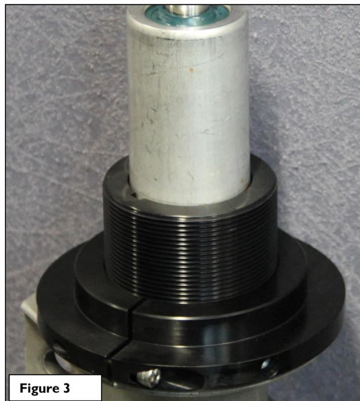
9. Install sleeve clamp as shown, aligning the notch in the clamp with the notch in the threaded sleeve. Secure sleeve clamp screw using the supplied 4-40 screw until snug. The clamp prevents the sleeve from turning when adjusting ride height. See Figures 4 & 5.
