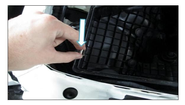
11. Install the Dinan spring clips into the lower airbox. The lower airbox should look like this:
