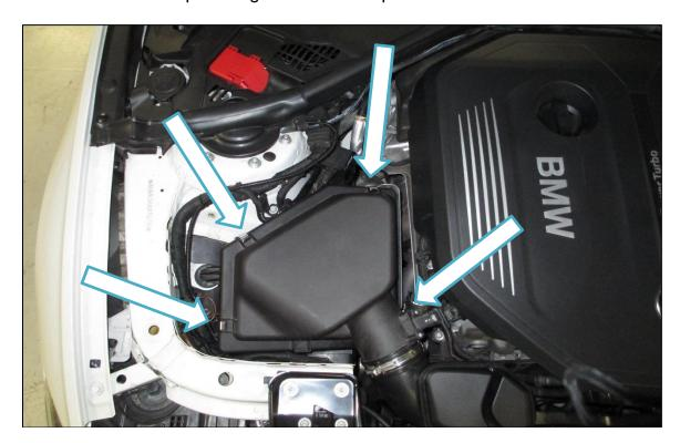
5. Follow the outlet of the airbox, down to the hose clamp near the turbocharger inlet. Loosen this hose clamp. A long extension and universal joint would be very helpful with this step.
