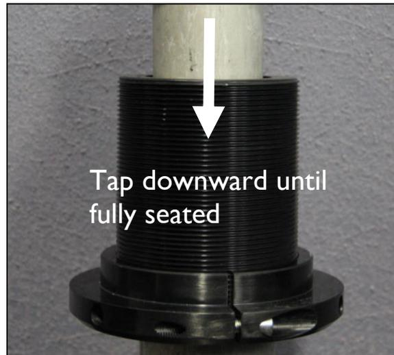
7. Verify that the sleeve has fully seated onto the shock. Measure the distance between the top of the shock and the threaded sleeve as shown below. When fully seated, your measurements would be:
