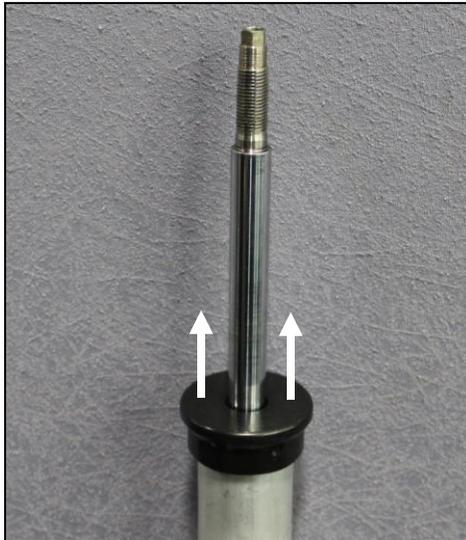
5. Remove spring perch plate. Wrap shock in towel and place in vice. Gently tap perch plate toward top of shock with hammer/mallet until it comes loose.
