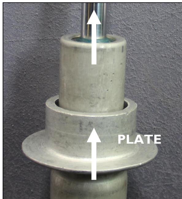
6. Install the Dinan Threaded Perch Assy. This part is a press fit. Use the same procedure as removal of perch plate for install. Take care to prevent damage to the threads!
