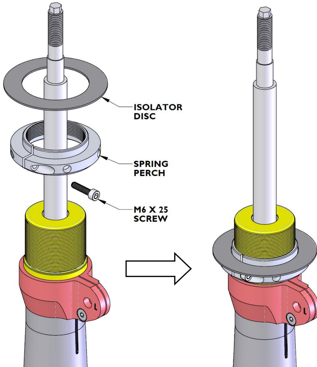
13. Install the rest of the front strut components as shown.
