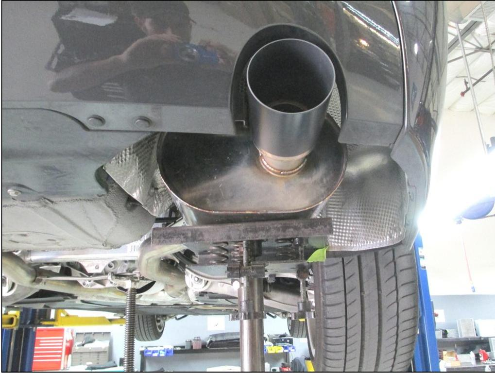
6. With muffler held in place, tighten front and rear hangers, torque to **15 ft-lbs (21 Nm)**.
