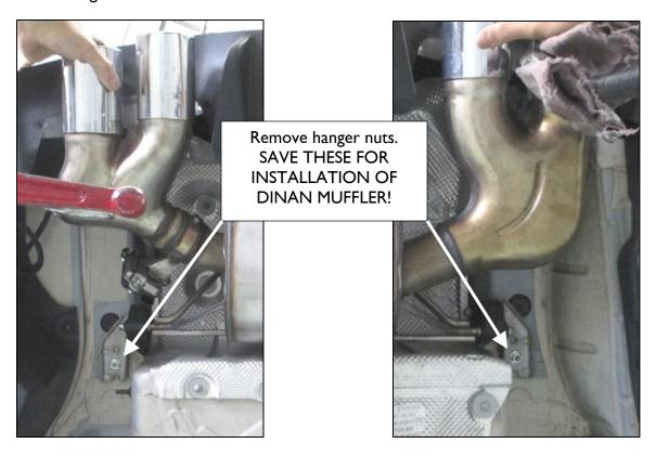
5. Remove both hangers and valve actuator from stock muffler. SAVE THESE PARTS FOR INSTALLATION ON DINAN MUFFLER.
