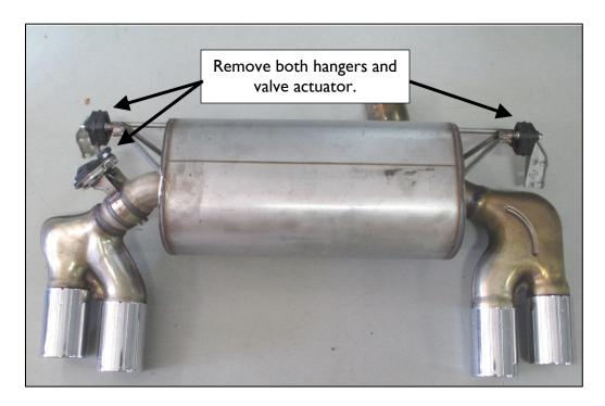
6. There are two types of DINAN exhaust valves. Examine the following diagrams to determine which type is on your DINAN exhaust. Using the hardware provided, install the valve actuator mounting brackets, as shown in the appropriate diagrams.
