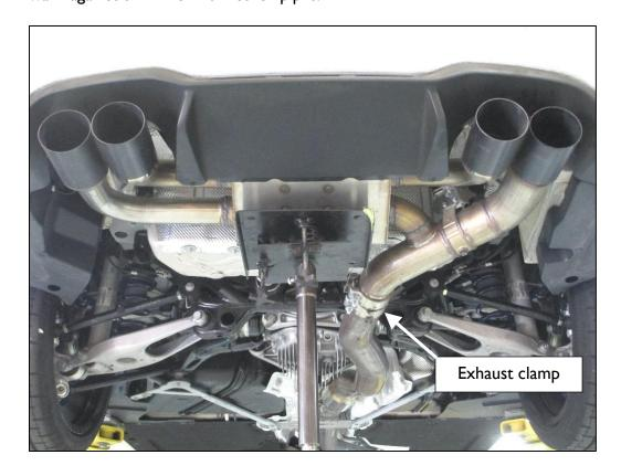
11. Mount both muffler hangers using the stock mounting nuts that were saved from removal of the stock muffler. Torque the nuts to 14 ft-lbs (19 Nm).
