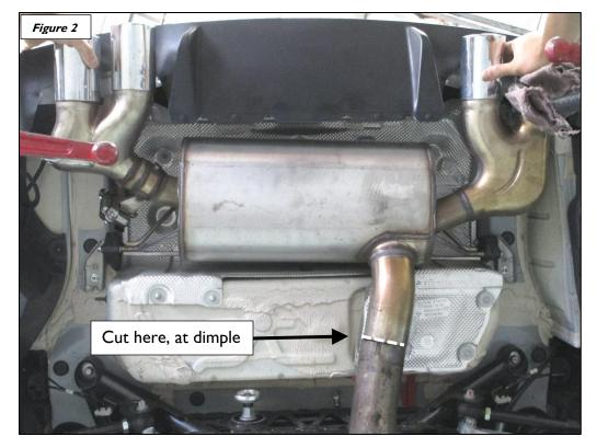
4. With the stock muffler fully secure and supported on a jack or stand, remove the hanger nuts as shown (SAVE THESE NUTS FOR INSTALLATION OF DINAN MUFFLER!), then remove stock muffler. Be sure exhaust valve actuator is disconnected before finally removing the muffler.
