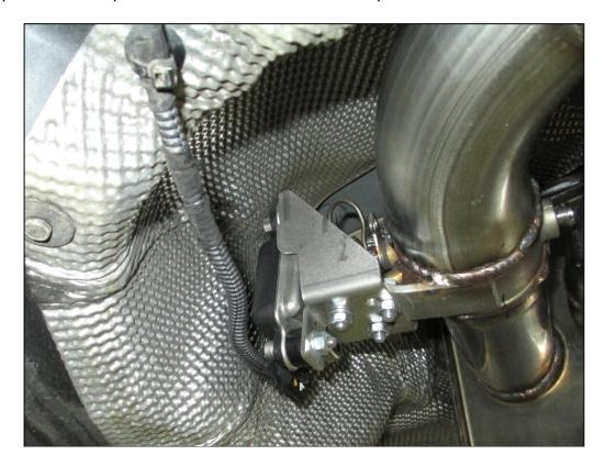
19. The passenger-side harness is too short. Again, cut the factory zip-tie. Pull the plug and route it through the valve motor mount bolts and plug it in as shown below. Reinstall a new zip-tie to prevent the harness from drooping. Cut off the excess tail on the zip-tie.
