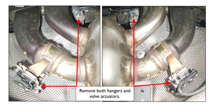
6. Install the valve actuator mounting brackets provided in the hardware kit as shown below. You will need (3) M6x20 bolts, (3) M6 locknuts, and (6) M6 washers from the hardware kit provided to install each mounting bracket. Notice the location of the spacer for mounting the actuator in the next step. Make sure all hardware is tight.
