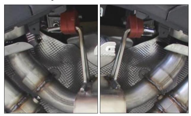
9. Place exhaust clamps provided in the hardware kit onto the inlet ends of the muffler. With DINAN exhaust secured on a jack or stand, rotate the muffler into place by positioning the outlet tubes into the tips attached to the bumper, then rotate the muffler inlet tubes up to mate to the stock tubes. Slide the clamps over the tubes and push the muffler forward against the ends of the stock pipes.
