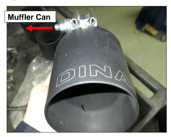
14. Slide the tip over the outside outlet tube as far as it will go. Hold the tip steady, with a finger gap between Top Dead Center (the 1<sup>st</sup> "N" in DI**N**AN") and the bumper. Use a 15mm socket to tighten until snug on the muffler, but still allows for final adjustment. Check to confirm there is approximately 1/8" protruding beyond the bumper at TDC (see below), then fully tighten.
