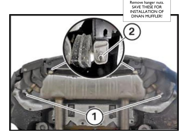
5. Remove both hangers and valve actuators from stock muffler. SAVE THESE PARTS FOR INSTALLATION ON DINAN MUFFLER.
