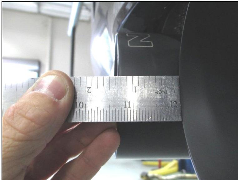
16. Check the exhaust tips for proper bumper clearance and proper alignment.
