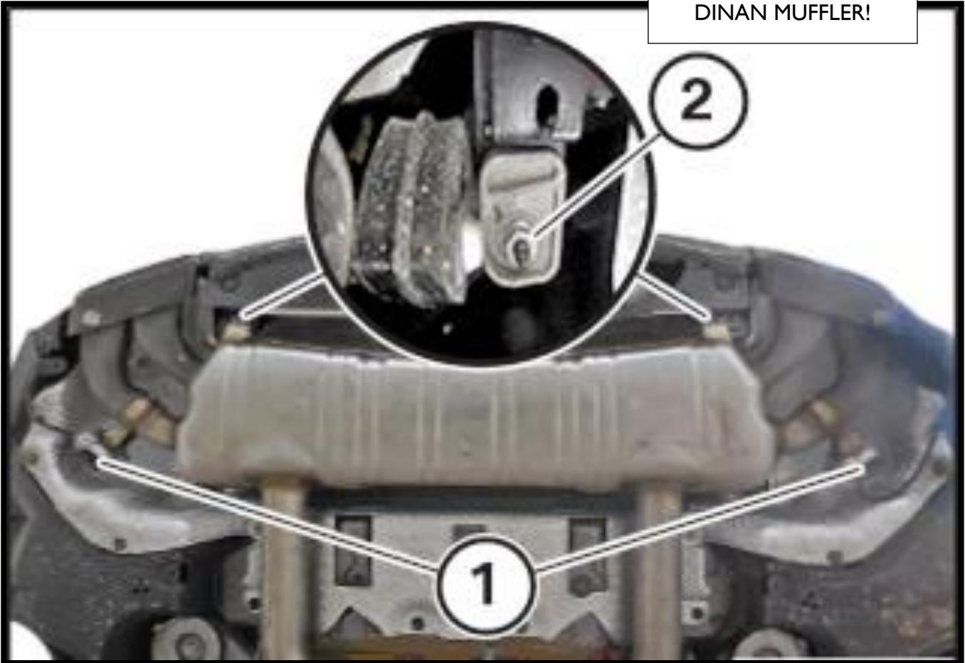
5. Remove both hangers and valve actuators from stock muffler. **SAVE THESE PARTS FOR INSTALLATION ON DINAN MUFFLER.**
