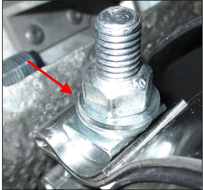
13. The clamp must have the nut facing the muffler when installed on the car. Slip the clamp over the slotted flange at the back of the tip with the screw / nut on top, parallel with the Dinan logo, as shown below. Tighten the clamp until it is snug on the flange, while still allowing side-to-side rotation.
