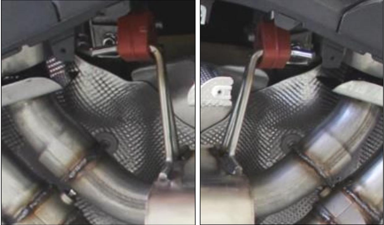
9. Place exhaust clamps provided in the hardware kit onto the inlet ends of the muffler. With DINAN exhaust secured on a jack or stand, rotate the muffler into place by positioning the outlet tubes into the tips attached to the bumper, then rotate the muffler inlet tubes up to mate to the stock tubes. Slide the clamps over the tubes and push the muffler forward against the ends of the stock pipes.
