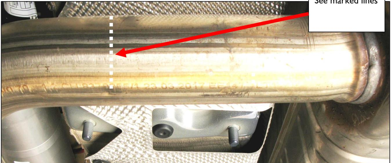
4. With the stock muffler fully secure and supported on a jack or stand, remove the hanger nuts as shown (SAVE THESE NUTS FOR INSTALLATION OF DINAN MUFFLER!), then remove stock muffler. Be sure exhaust valve actuators (1) are disconnected before finally removing the muffler.
