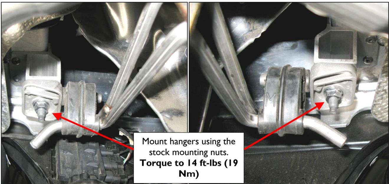
11. With exhaust clamp rotated as shown, torque clamps.
