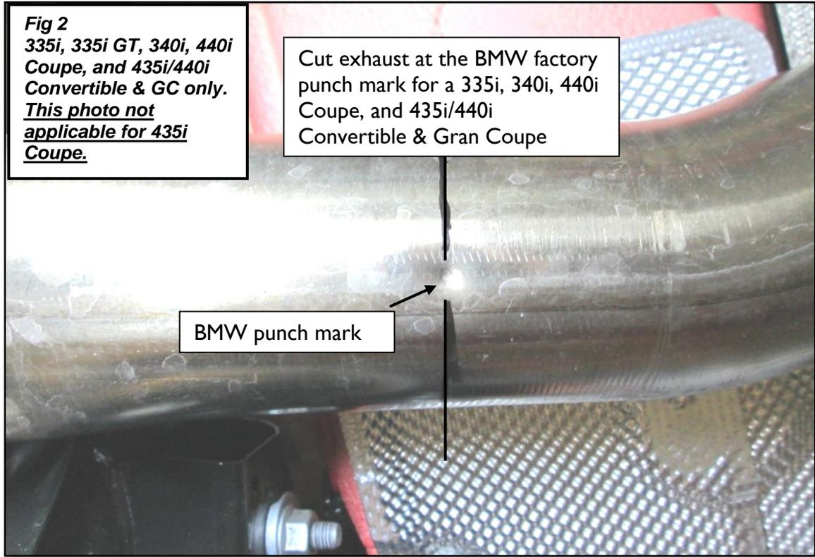
3. Support the stock muffler with a jack or stand. See figure 3. Use a Sawzall or similar cutting tool.
