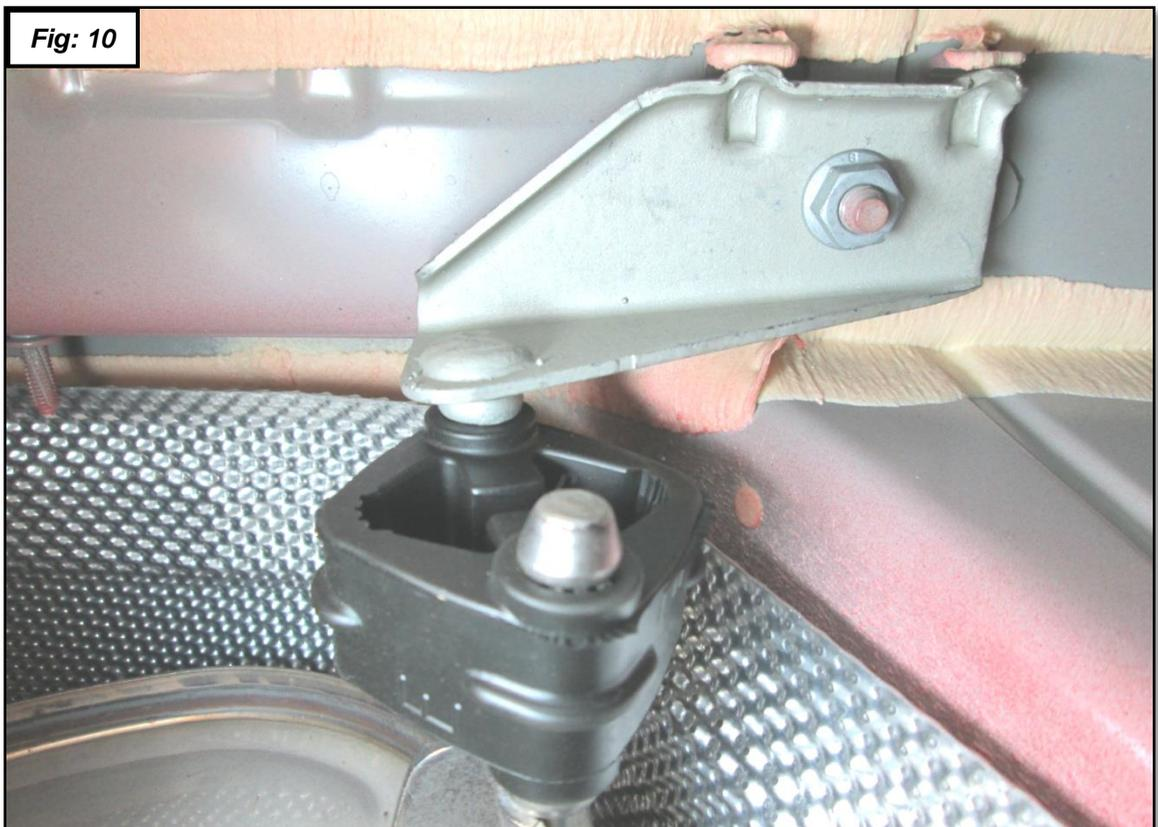
9. Transfer muffler hangers to new mufflers as shown in figures 11 and 12.
