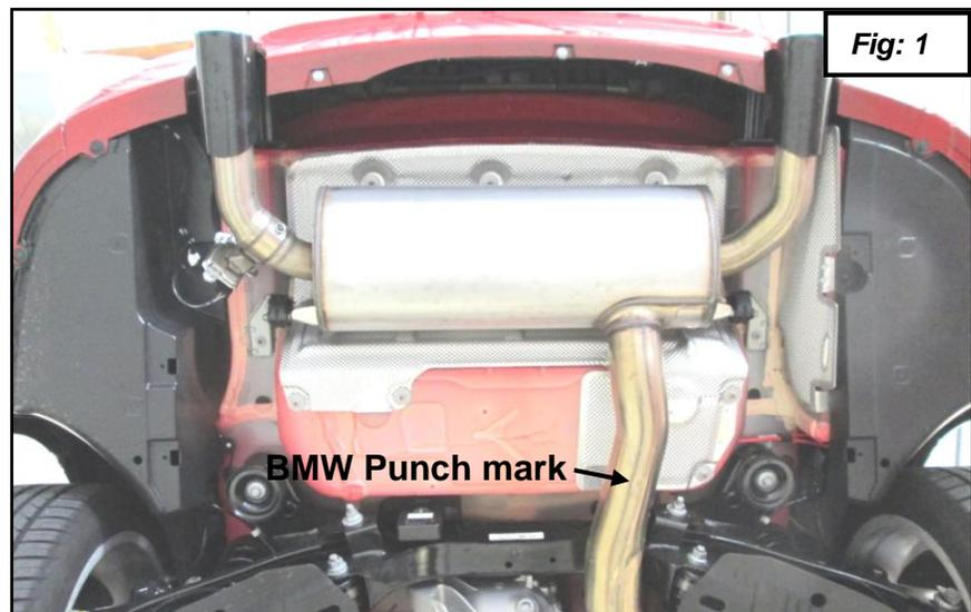
2. This step applies to F22/F23 M240i, F30/F34 335i/340i, F32 440i Coupe, F33 435i & 440i Convertible, F36 435i & 440i Gran Coupe only; skip to step #4 if you are working on a F32 435i Coupe. For a M240i/335i/340i/440i Coupe/435i Convertible & Gran Coupe, cut off the stock muffler at the punch mark as shown in figures 1, 2, and 3. Mark the cut line.
