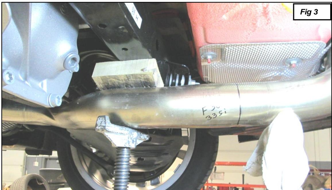
4. **This step applies to F32 435i Coupe only; skip to step #6 if you are working on a F22/F23 M240i, F30/F34 335i/340i, F32 440i Coupe, F33 435i/440i Convertible, or F36 435i/440i Gran Coupe.** For a 435i coupe, find the BMW factory punch mark on the exhaust. Measure  $\frac{3}{4}$  of an inch from the punch mark toward the back of the car and cut at that point.
