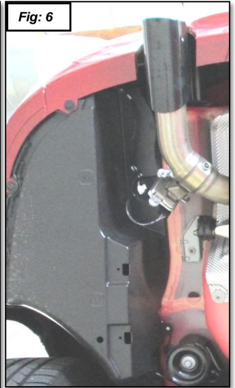
7. Remove the 3 screws and 1 nut holding the left inner body side cover and let it hang down to give you access to a spot to zip tie the valve out of the way as shown in figure. Position the actuator with the wire connector down and the shaft pointing to the inside as shown. Reinstall the side cover. See figure 8.
