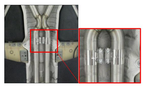
14. The driver's side inlet pipe requires additional attention. There is minimal clearance between the pipe and the underside of the car, near the transmission brace. Adjust the pipe to maximize the clearance in this area, as shown in the following photos.
