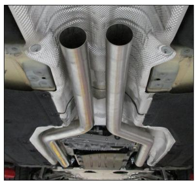
9. Slide the Dinan clamps onto the inlet pipes, with the hardware towards the middle of the car, as shown below.
