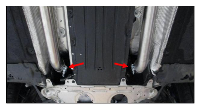
7. Push each pipe forward up against the lip, so that there is NO gap between the Dinan pipe, and the outlet from the engine.
