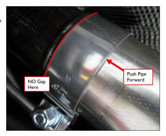
8. Tighten the clamps just enough to hold the pipes into place, but still allow some adjustment. Rotate the pipes until the preferred position is attained.
