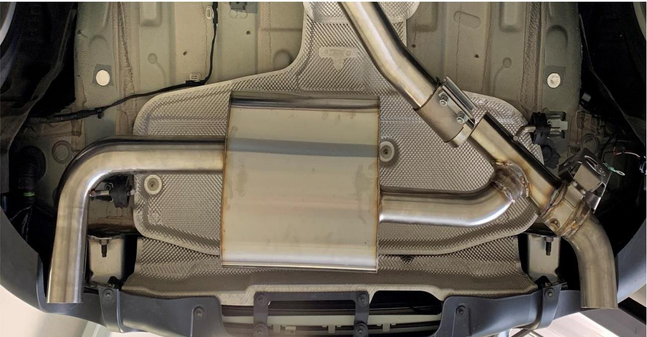
5) Slide the coupler clamp on, push up on the exhaust and toward the front of the car, and lightly tighten the coupler clamp.
