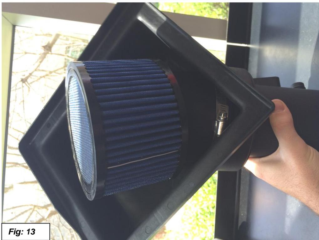
18. Test fit upper air box lid on lower air box to make sure that the filter orientation is not causing misalignment between the air boxes. Rotate filter as necessary to clear lower air box. Once the correct orientation is found, tighten clamp with 8mm wrench.
