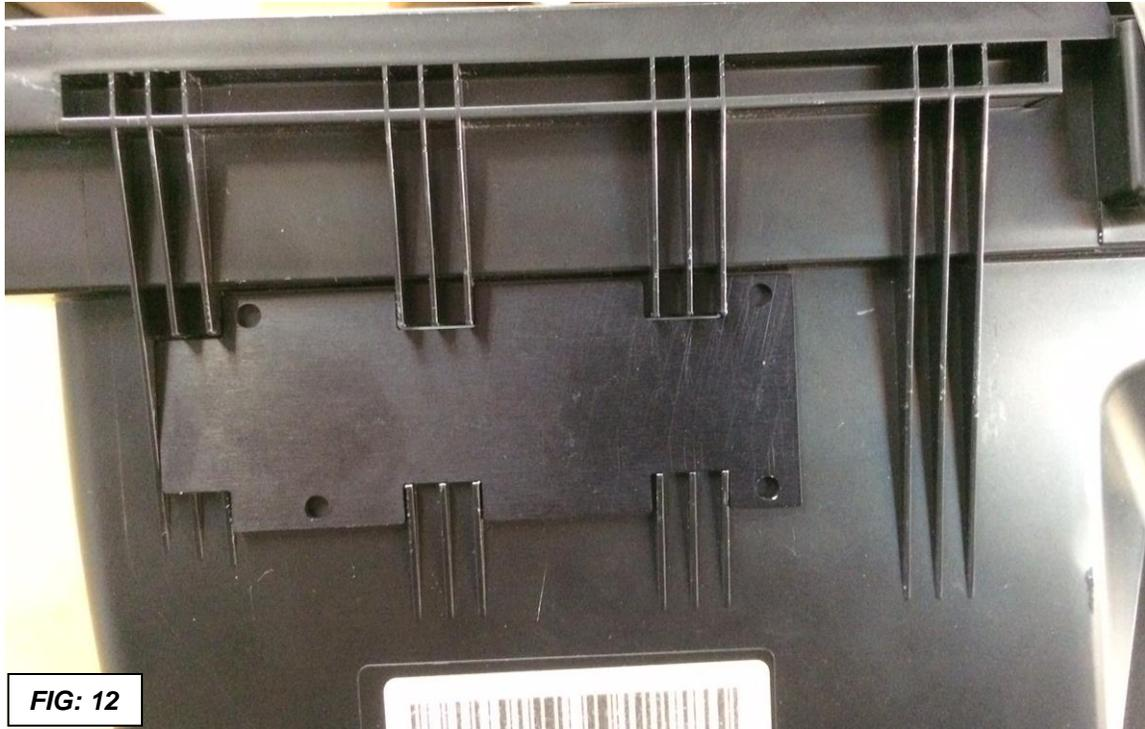
14. Using the cover plate as a drill template, drill the four hole pattern into the airbox using a #30 size drill bit. Install the 4 blind rivets in the hardware kit from the outside of the airbox.
