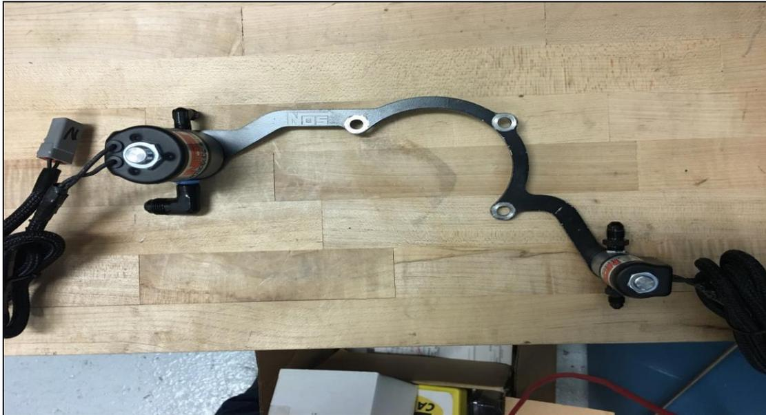
**Figure 6 – Solenoid Bracket Assembly**
