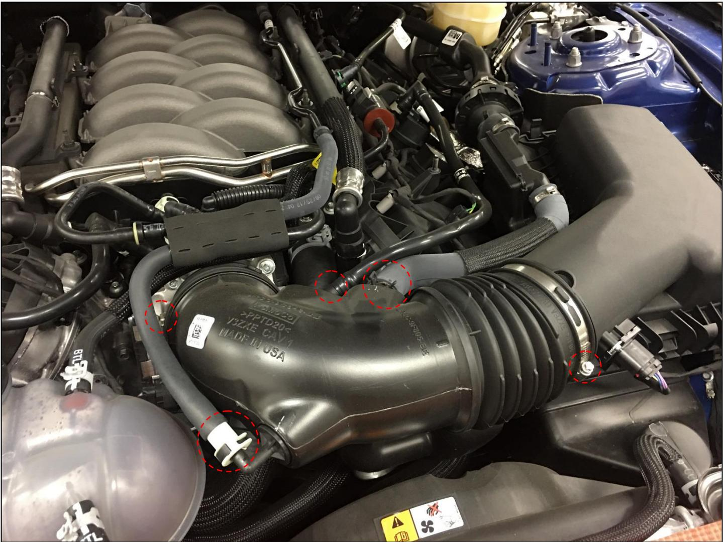
**Figure 8 – Intake Air Tube Removal**
