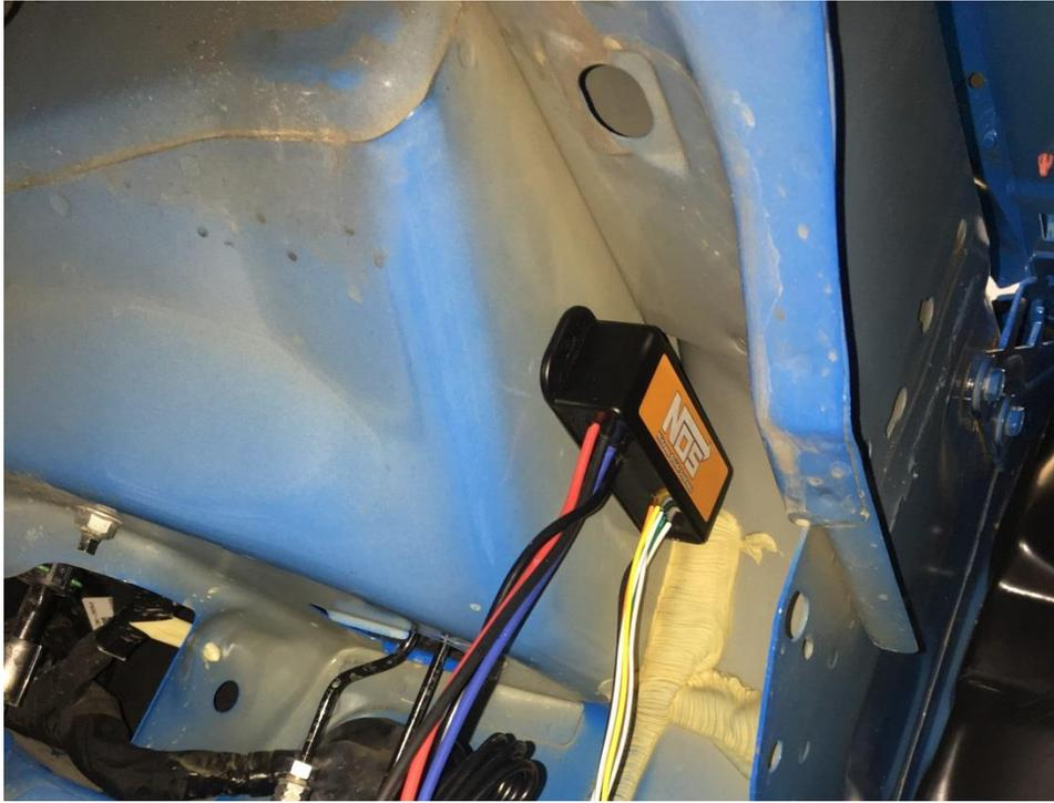
**Figure 16 – Mini 2-Stage Mounting Location**
