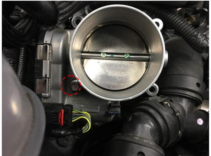
7. Install the solenoid bracket and solenoids assembly you built in section 2.4 to the outside diameter of the throttle body with the three remaining, longer throttle body screws as shown in **Figure 10**. **Do not tighten completely.**
