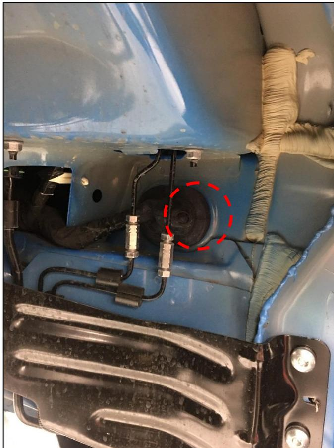
**Figure 17 – Wiring Pass Through**
