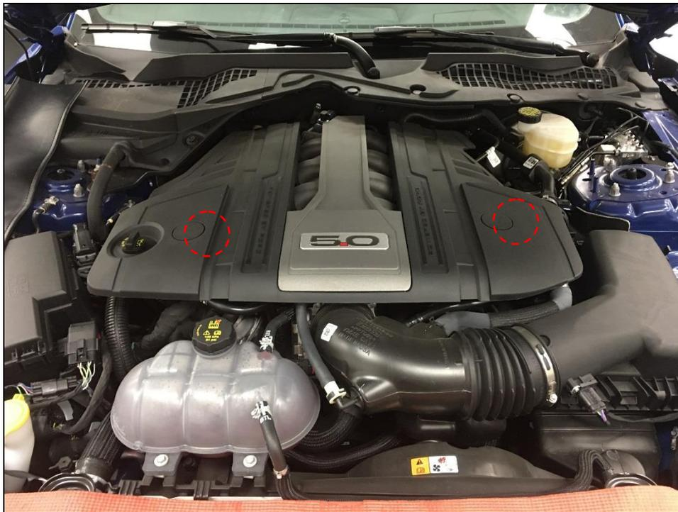
**Figure 7 – Engine Cover Removal**
