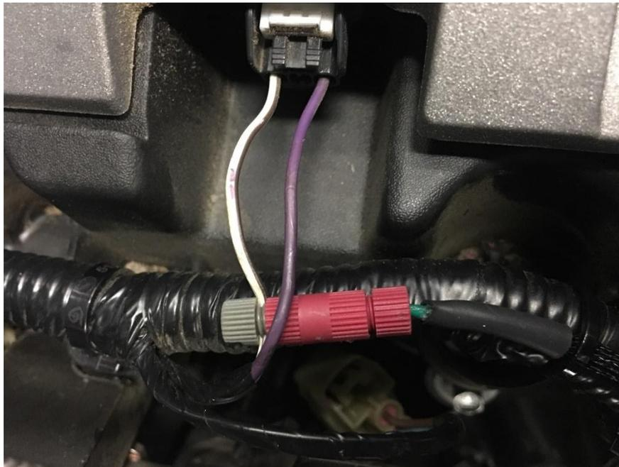
**Figure 18 – Tach Signal Wire Connection**
