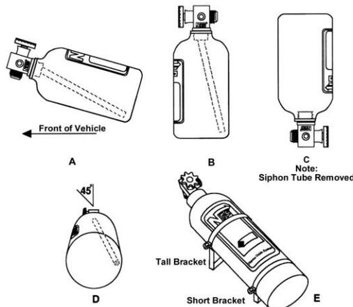
Figure 3 Nitrous Bottle Mounting Orientations
