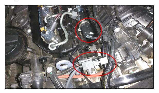
\*\* NOTE: Some E90 335d and E70 X5 vehicles were equipped with an alternate sensor, and the connector on the DINANTronics SPORT harness will not plug in. If this is the case with your vehicle, simply remove the "key" inside the DINAN plug, which will allow a connection with the sensor.
