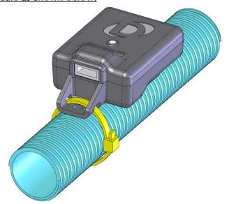
7. Mount the module at the location shown below. Use a zip-tie to secure the harness as shown. Also ensure adequate slack in the wiring harness to allow for engine movement. It is best to orient the module vertically, with the wiring pointing downward.
