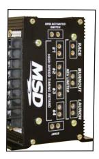
Racer input was garnered about the features of the new PN 7330 and MSD listened. The start retard is now adjustable, the four retard stages activate from +12 volts and the ignition can be used on 4, 6 or 8-cylinder engines.
