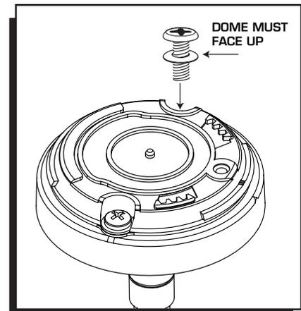
Figure 2 Washer Installation.
