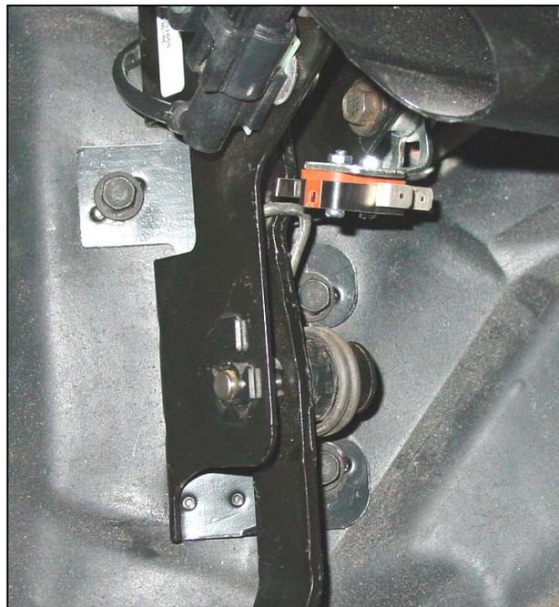
**Figure 16 Microswitch in completed location**
